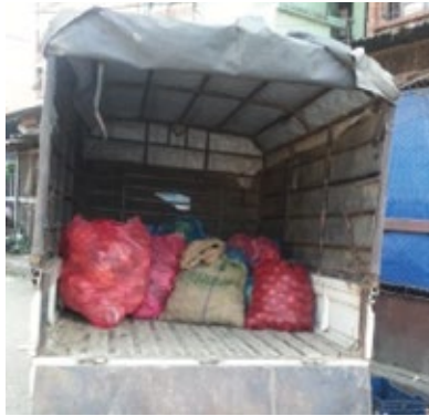
Transport vehicle with light-colored cover absorbs less heat.
