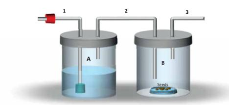
Figure 1.5. Humidity (water content) adjustment in seeds. The system for adjusting seed moisture (water content) uses flow-through chambers. The gas (or air) to be humidified) flows through tube 1 into the glycerol-water solution in jar A. The humidified gas then flows through tube 2 into the controlled-environment chamber (jar B) and exits into the atmosphere through tube 3. (Modified from Forney and Brandl, 1992).
