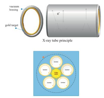
X-ray tube (centre) surrounded by orbiting and rotating sample canisters.
