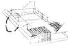
Industrial shellfish dredge Weight 500-1000 kg
