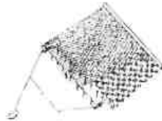
Dredge with teeth, on the lower edge of the frame and with depressor flap on the upper edge Weight 70-100 kg
