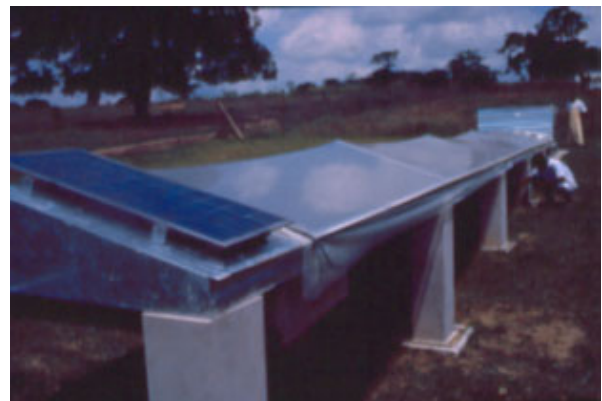
Fig. 293: Higher-cost construction of tunnel dryer. Roof-shaped solar collector, top part made of metal frames and bottom part made of metal-coated polyurethane panel. Length 15m. (Type 2 in table 13).
