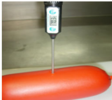
Fig. 120: Large calibre sausage upon heat treatment (core temp. +70.3°C) (see also table 8, page 142)
