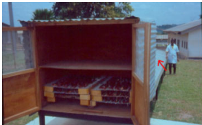
Fig. 294: Drying chamber (made of wood) connected to solar collector (arrow) of tunnel dryer. Trays with meat to be dried positioned in the chamber
