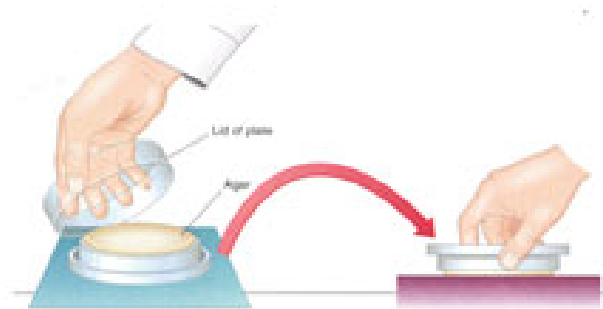
a) Impression on test surface (purple colour). Direct transfer of bacteria from test surface to culture medium (in petridish)
