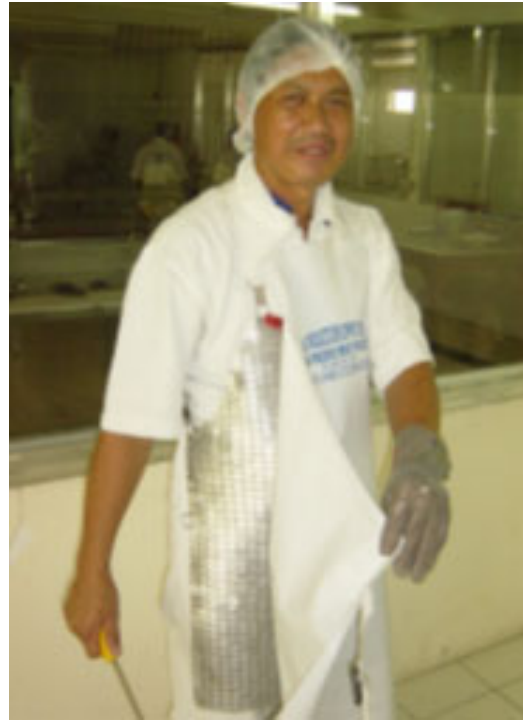
Fig. 409: Protective appliances: anti-cut glove and apron (should be worn under the plastic apron to avoid contact with meat and fat pieces)
