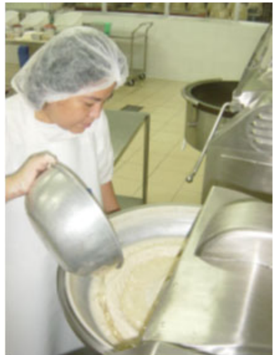
Fig. 95: Preparation of milk protein/water/animal fat emulsion
