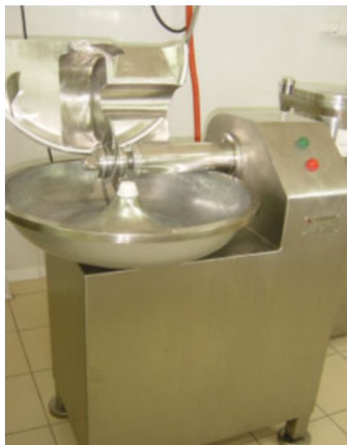
Fig. 312: Bowl cutter (18 litres) single phase power
