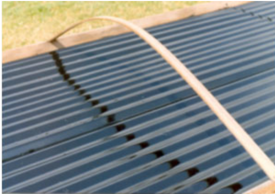
Fig. 290: Simple construction of low-cost solar collector. Bottom part made of black painted corrugated steel plate. Wooden rafter as support for the transparent plastic film to cover the collector
