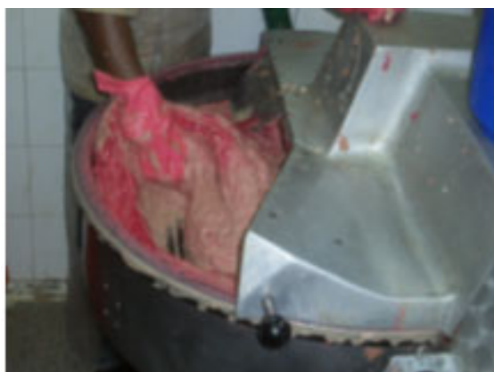
Fig. 101: Addition of red food colourings during comminuting of batter for raw-cooked meat products
