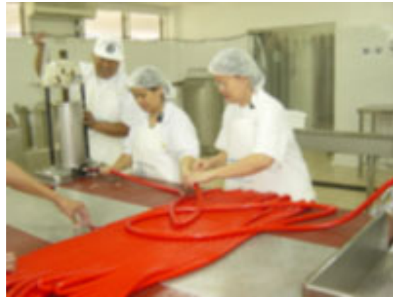
Fig. 327: Product in red coloured cellulose casings (cal. 22) used to transfer colour to sausage surface
