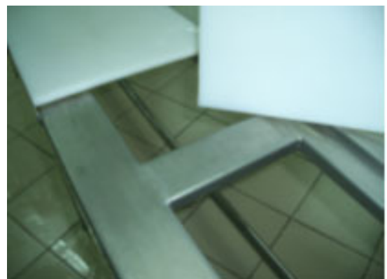
Fig. 484: Meat cutting table, frame made of stainless steel, plastic boards removable for easy cleaning
