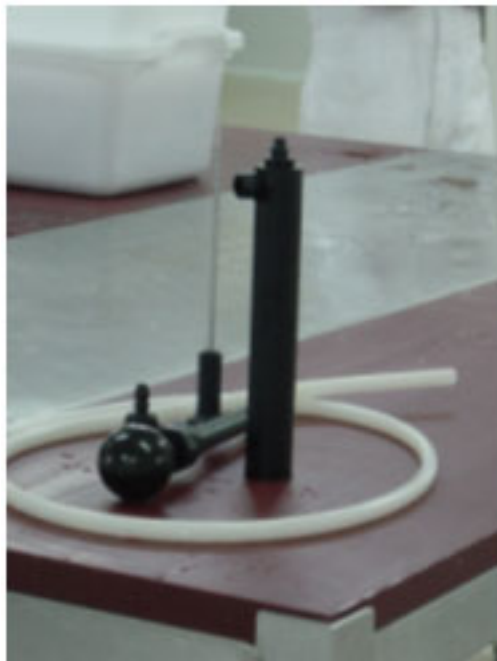
Fig. 93: Application by injection of additives in watery solution; pump and injection needle for brine (see also Fig. 226)
