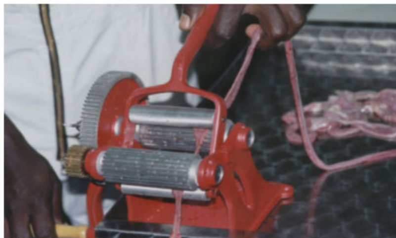
Step 3: Loosening of tissue layers using a small-scale manual casing cleaning machine
