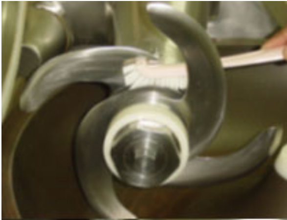
Fig. 399: Gap between bowl and knife shaft.
