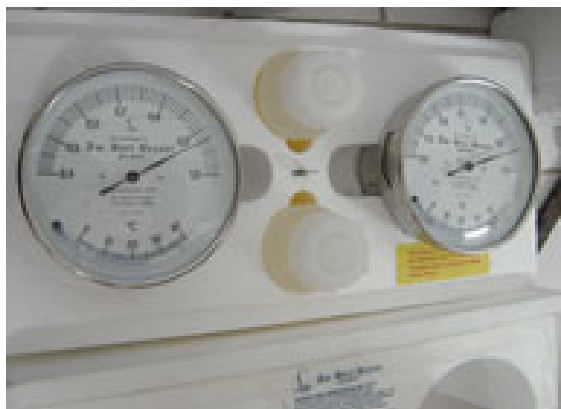
Fig. 427: Set of two simple a_w -meters enabling simultaneous measurements of two samples
