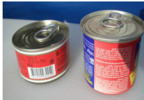
Fig. 371: Two-piece cans. Left steel can, right aluminium can. Steel can be shallow drawn, aluminium can be deep drawn
