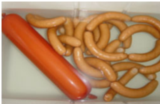
Fig. 178: Immersion cooling: The smoked and cooked products are cooled down in cold water
