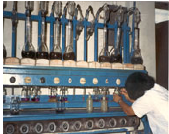
Fig. 435: Kjeldahl distilling apparatus (for protein)
