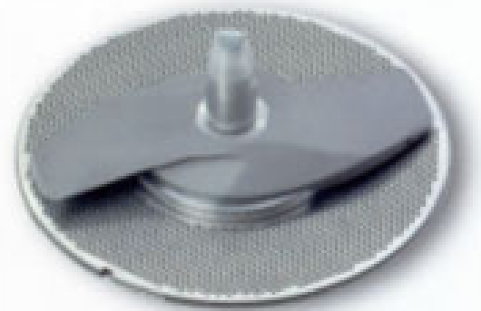
Fig. 55: Emulsifying machine (plate and rotating blade)
