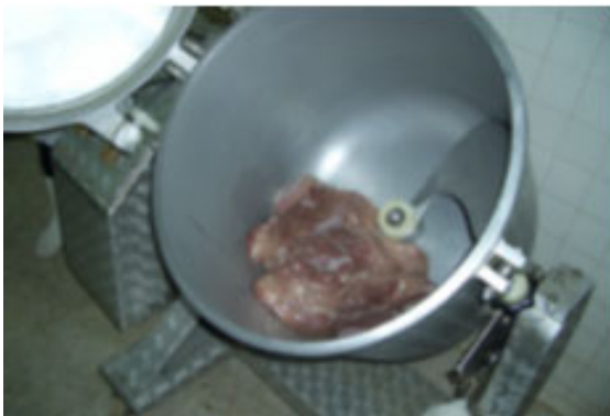
Fig. 228: Tumbling of pork pieces, brine added to tumbler
