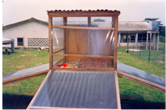
Fig. 296: Drying chamber of multi-collector dryer. Front and side walls of the chamber are transparent to collect additional solar energy. Air inlet from collector to chamber
