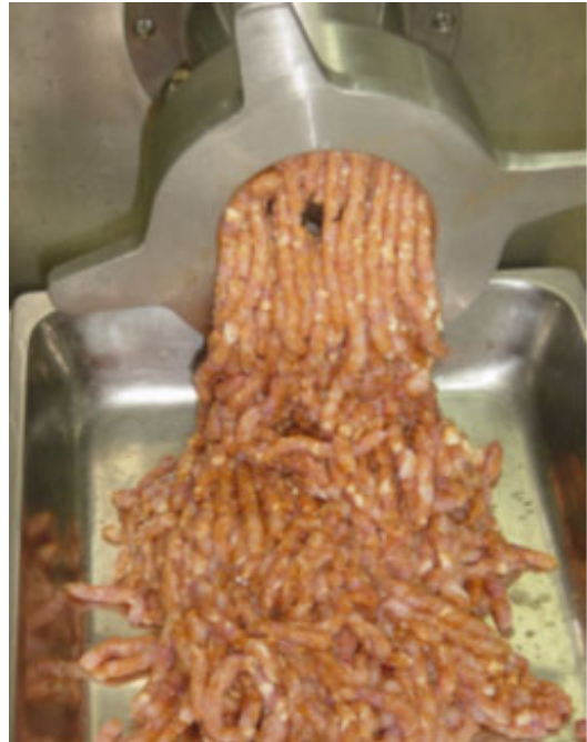
Step 1: Mincing of meats to be added to finely chopped batter for coarse sausage
