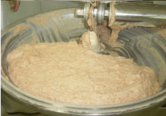
Step 2: Coarse material is added to finely chopped batter (above). Final mixture after a few rounds in the bowl cutter (below)
