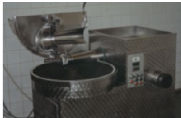
Fig. 29: Bowl cutter–grinder combination (twin model) with bowl cutter (60 litres capacity) and meat grinder (114 mm orifice diameter)
