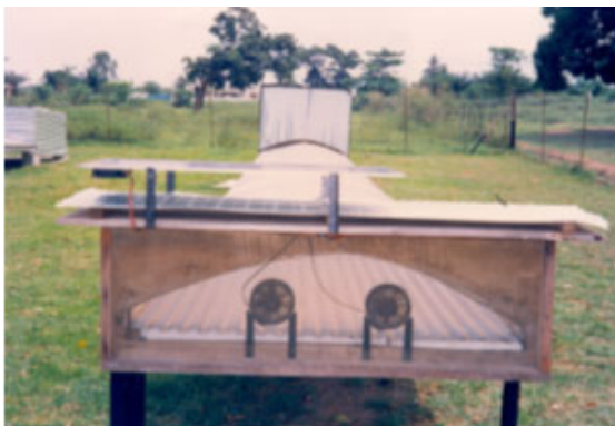
Fig. 292: Functional simple solar tunnel dryer. Front part of solar collector with air inlet and two electrical fans for reinforcement of air stream. Photovoltaic panel on top of the front part to drive the fans. Collector with corrugated bottom metal sheet and transparent foil cover. Length of solar collector 11.5m. Drying chamber located at the end of the solar collector. (Type 1 in table 13).
