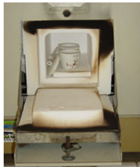
Fig. 437: Muffle furnace (for minerals)
