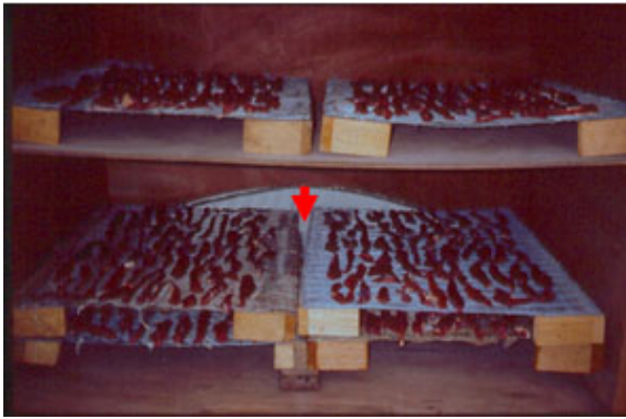
Fig. 295: Air inlet (arrow) from the solar collector (tunnel type) into the drying chamber
