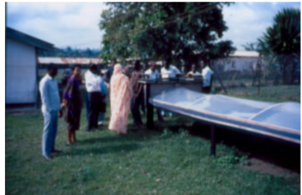
Fig. 291: Completed simple solar collector, covered with transparent UV resistant plastic sheet
