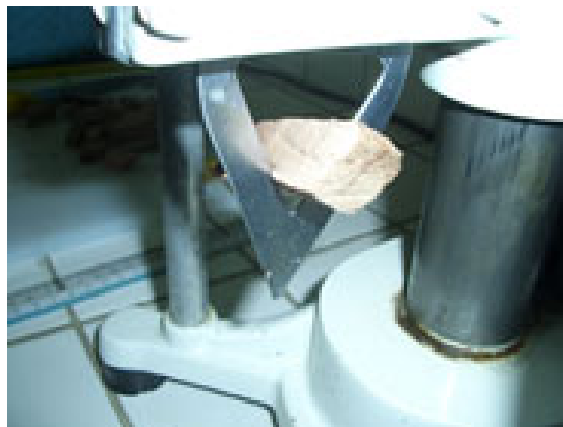
Fig. 433: Measurement of shearforce
