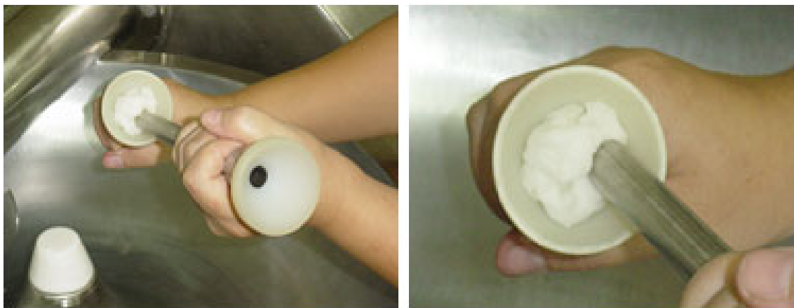
Fig. 402: Simple method to retrieve sausage batter from funnels before cleaning by means of a paper towel
