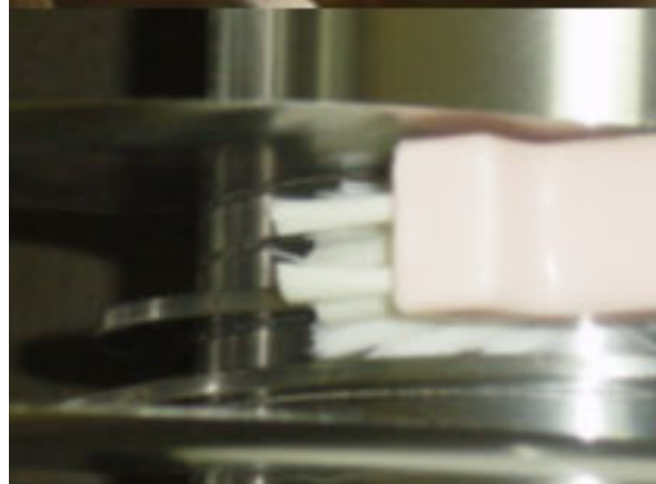
Fig. 398: Cleaning of spaces between knives with small brush
