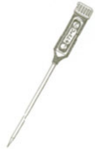
Fig. 421: Compact digital thermometer
