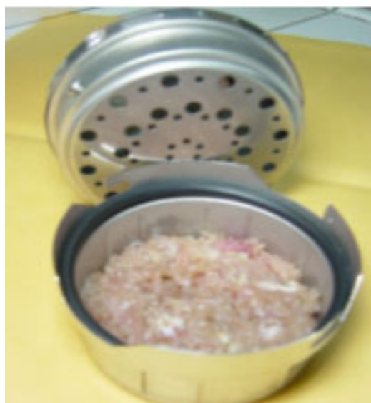
Fig. 428: A_w -meter with product sample to be tested, lid (has to be attached) with built-in hygrometer
