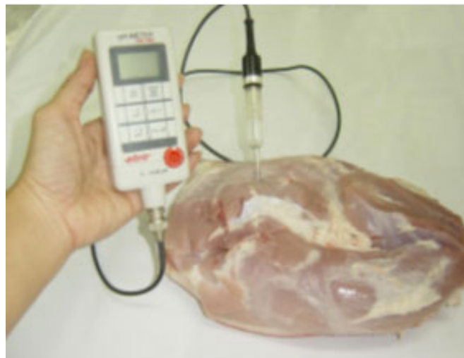
Fig. 222: pH – measurement in ham
