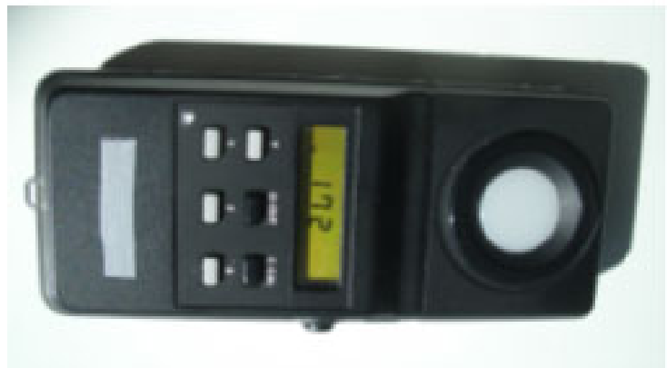
Fig. 431: Lux-meter Light sensor and monitoring unit in one portable instrument
