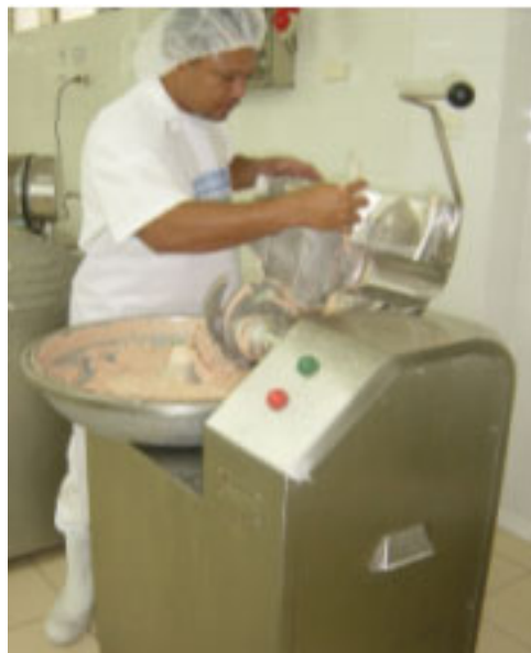
Fig. 59: Chopping of meat mixture in bowl cutter; lid opened after finalizing chopping, cutter knives visible
