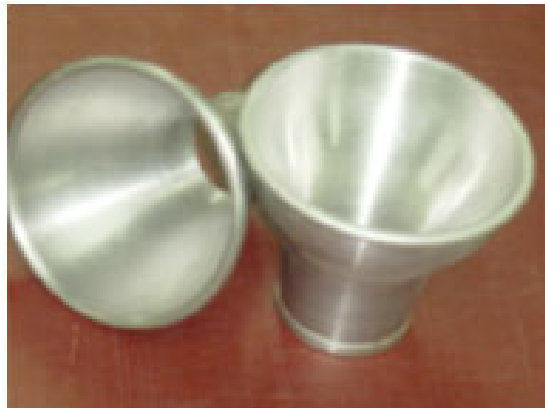
Fig. 412: Manual funnels for stuffing of larger calibre sausages, made of food-grade aluminium
