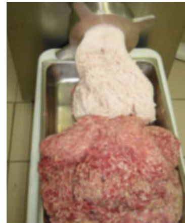
Step 1: Mincing of meat and fat (3 mm grinder disc)
