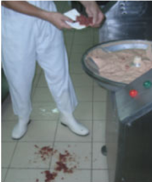
Fig. 470: Meat which falls accidentally onto the floor, must not be taken, goes to waste.
