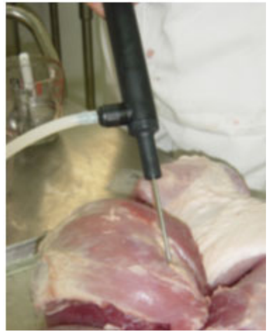
Fig. 67: Brine injection with a manual curing pump
