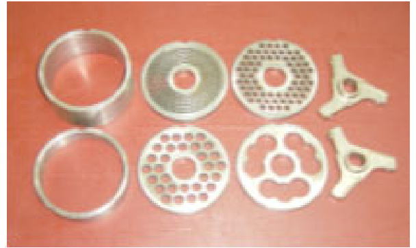
Fig. 21: Grinder plates of different hole size, star knives and spacer rings for tightening of cutting assembly
