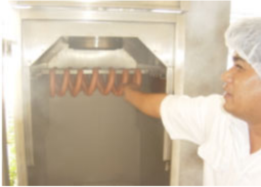
Fig. 174: All sausages are spread on a stick allowing smoke to circulate around each individual piece
