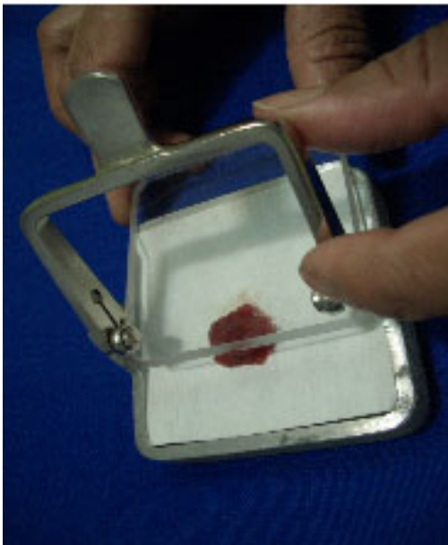
Fig. 429: Compressing meat samples for determination of water holding capacity
