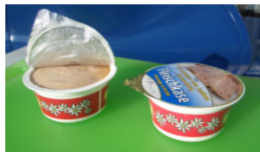
Fig. 374: Cans made of synthetic material with sealed aluminium foil as lid (can be torn off)
