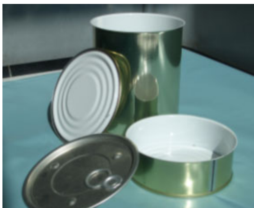
Fig. 370: Three pieces steel cans of different format, inside lining with synthetic compound, side wall induction soldered, lid with easy-to-open ring
