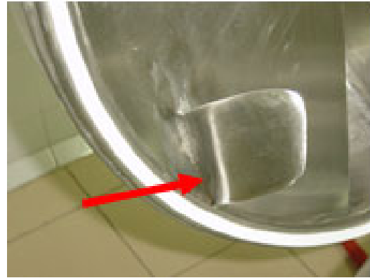
Fig. 400: Paddle on bowl cover with critical spot for cleaning
