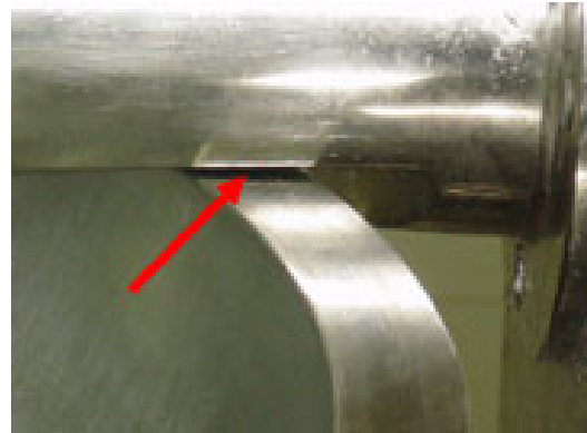
Fig. 399: Gap between bowl and knife shaft.
