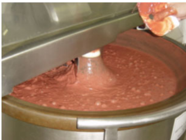
Fig. 190: Pre-chopping of raw liver (with curing salt). This batter is added later to the precooked hot meat materials (see Fig. 191)
