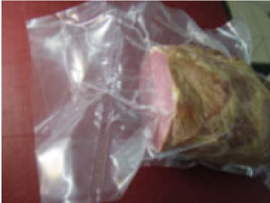
Fig. 347: Faulty sealing seam: risk of air penetrating inside the package because of film overlapping
