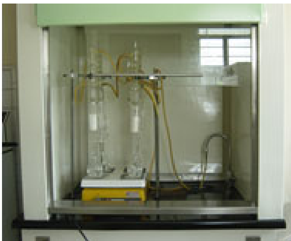
Fig. 436: Soxhlet extraction apparatus (for fat)
