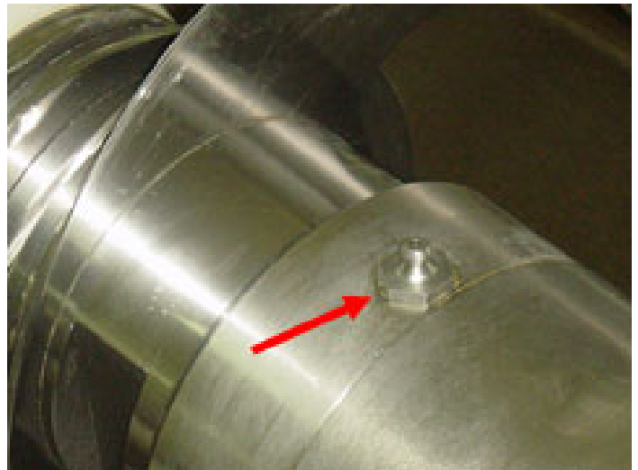
Fig. 397: Grease nipple on knife shaft housing
