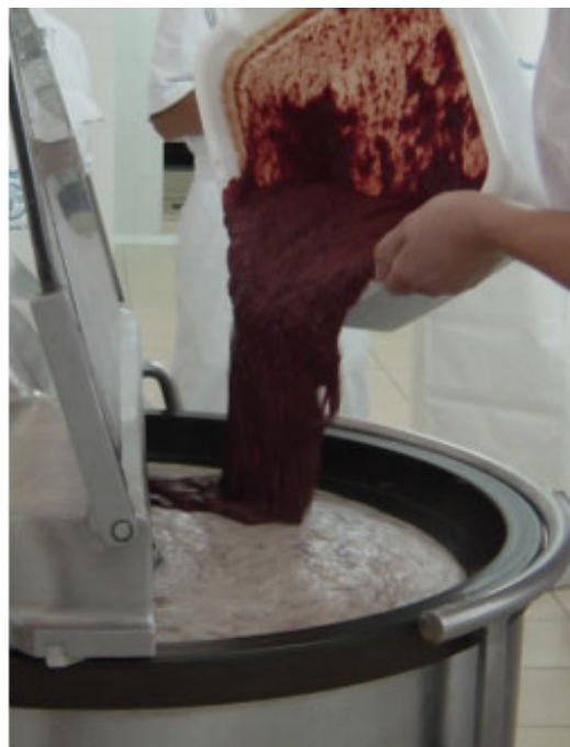
Fig. 191: Addition of chilled liver batter: The liver batter is added to hot precooked and pre-chopped meat materials in the bowl cutter. Bowl cutter is kept rotating in low gear.
