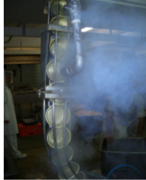
Fig. 375: Empty cans being cleaned by steam injection
