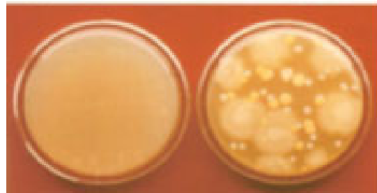
b) Testing of surface of meat processing equipment (above). Below left: Contact plate before impression. Below right: Contact plate after impression and incubation
