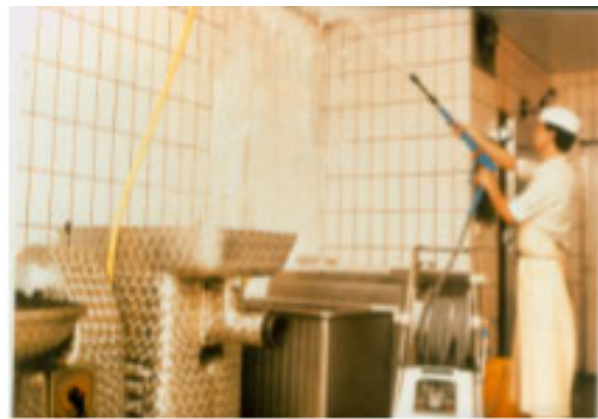
Fig. 489: Cleaning of wall with pressurized water - care must be taken not to contaminate equipment
