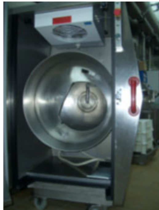
Fig. 49: Tumbler inside mobile refrigerated housing
