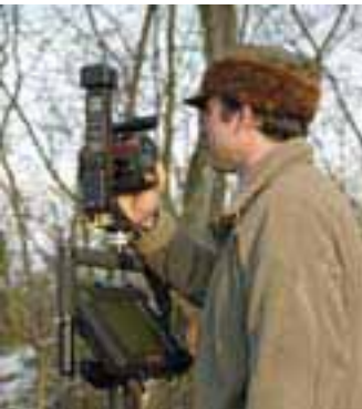
High-tech Czech hardware and software tool “Field-map” for tree mensuration and forest stand computation (www.ifer.cz)
