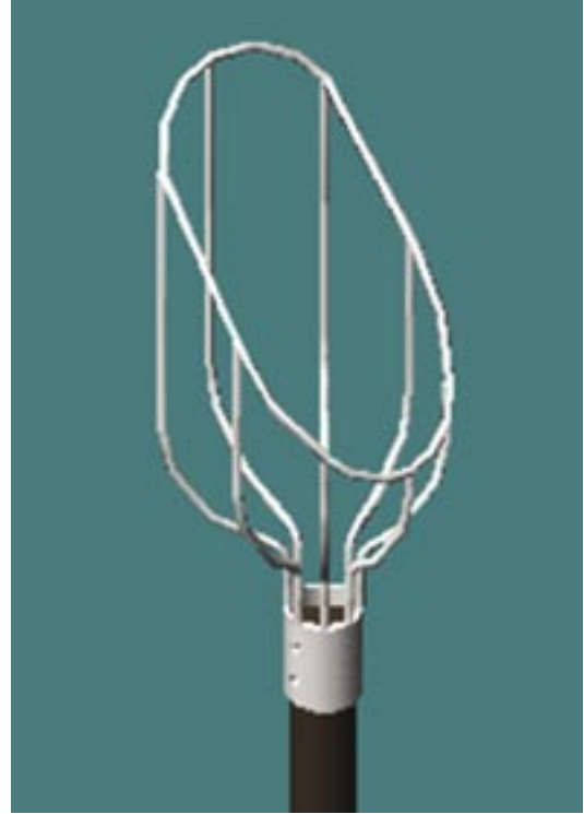
FIGURE 5 Harvesting tool for plucking of papaya (Design of the tool is given in Annex 2)
