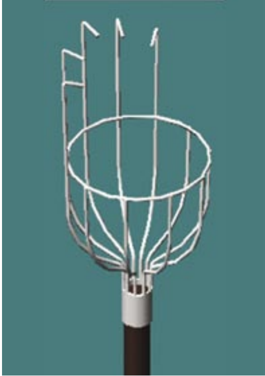
FIGURE 4 Harvesting tool for plucking of tree fruits occurring in bunches e.g. mango, avocado etc. (Design of the tool is given in Annex 1)
