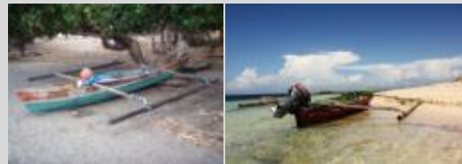
Type two. Boat made from a single piece of wood with panels attached. The simplest and cheapest version of this boat is without frames (left -Liquiça), although some are reinforced with frames (right -Atauro)
