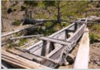
Big single bubur trunk boat with panels attached for fishing and with no frames. The photo shows the structure used to transport a large fish trap.
