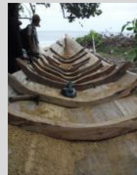
Wooden boat in Atauro, Bikeli. Presents a shallow freeboard (only 5cm from the waterline). Stem shaped in clipper style.
