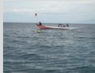
Wooden boat in Atauro, Bikeli. Presents a shallow freeboard (only 5cm from the waterline). Stem shaped in clipper style.
