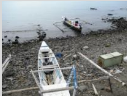
Type one. "Ro'o kik", made by a single piece of wood with paddles. With small outrigger (front) and without outrigger (back)
