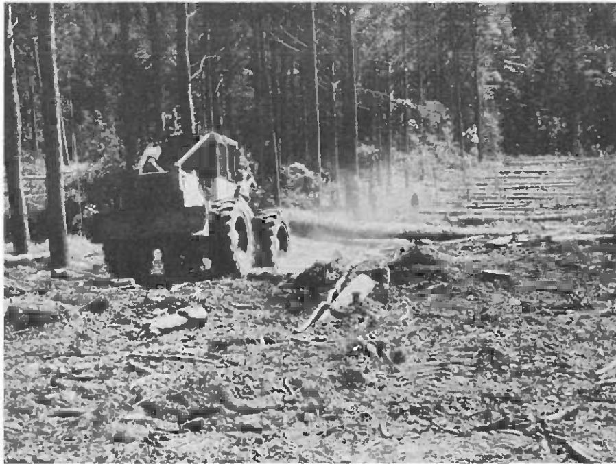
A CAT 518 rubber-tyred skidder in clearcut operation. The production was about 120 m 3 a day over an average skidding distance of 100 m. The logs were skidded in tree lengths and bucked at the roadside (Border Timbers Ltd.) (Photo: H. Seppänen)
