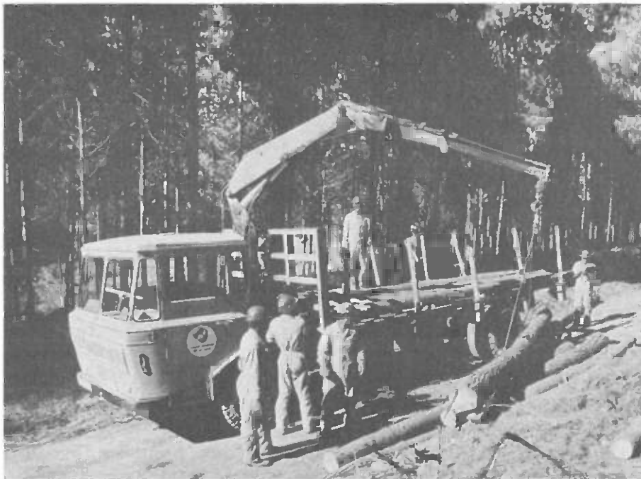
Logs being lifted by a truck-mounted self-loading loader using cable slings. The truck capacity was 8 m 3 . Logs were unloaded by releasing the truck stakes (Forestry Commission, Erin Estate) (Photo: H. Seppänen)
