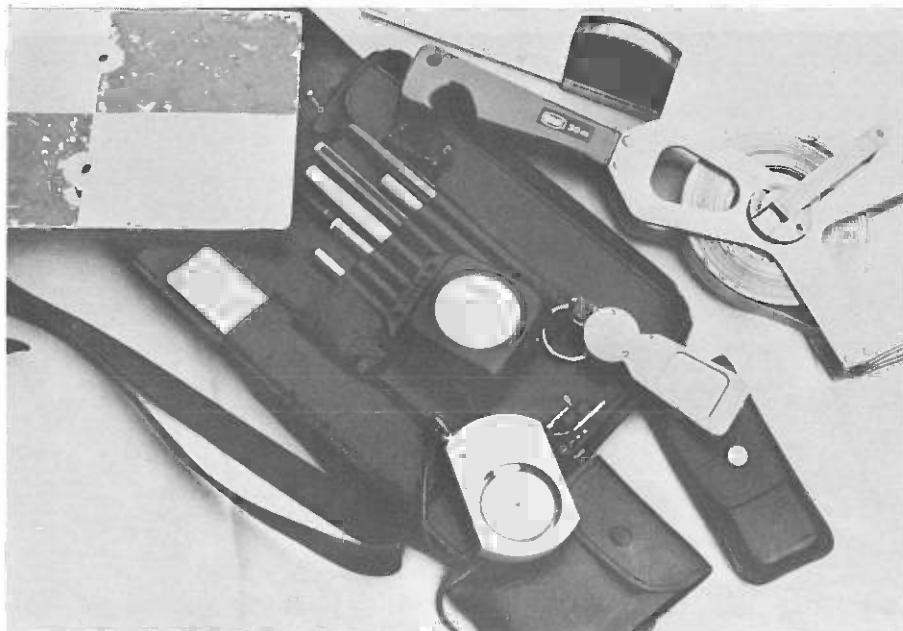
Engineer's wallet with instruments for road survey. (Photo: O. Sedlak)
