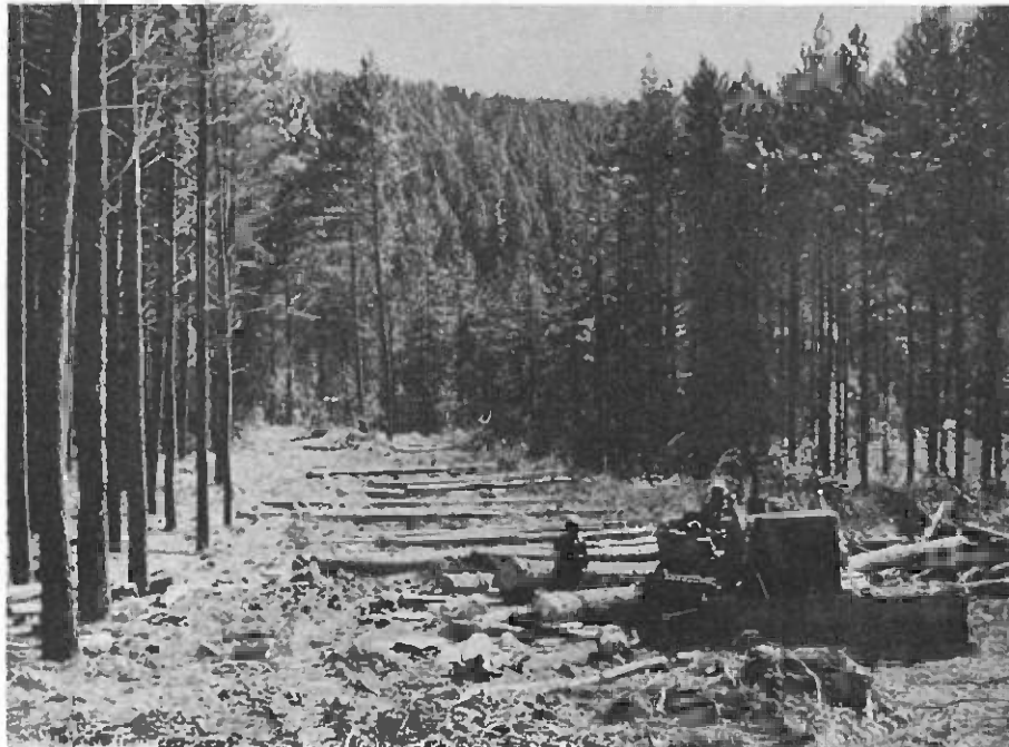
A CAT D-40 crawler tractor used in skidding Pinus taeda clearcut areas. The production was approximately 60 m 3 a day over an average skidding distance of 100 m (Border Timbers Ltd.) (Photo: H. Seppänen)
