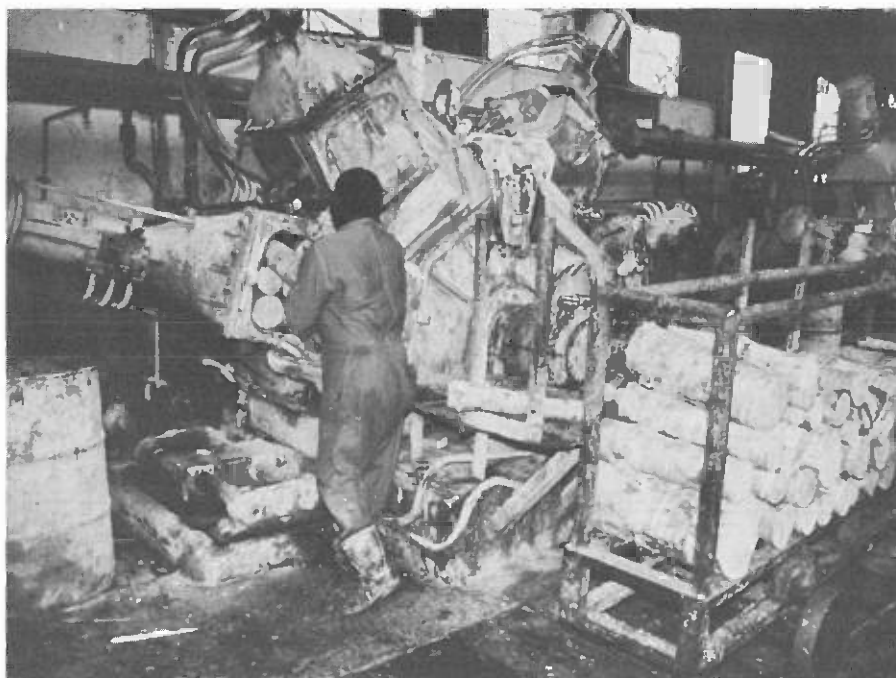
Loading a grinder in a pulp and paper mill (Mutare Board and Paper Mills) (Photo: H. Seppänen)
