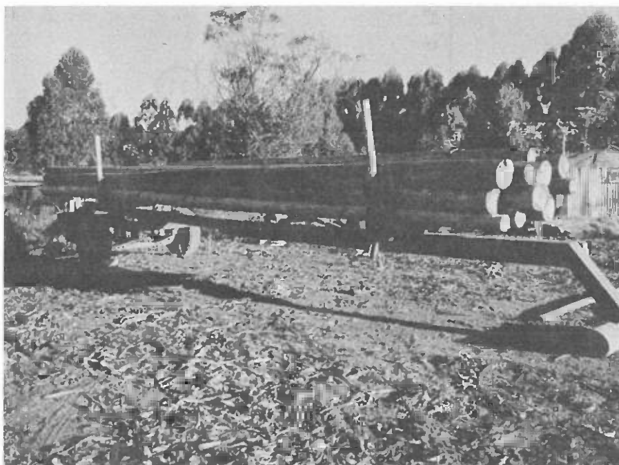
A unique trailer with rear-axle steering designed by the Wattle Co. Ltd. It was built to facilitate transport of long poles around tight curves on steep terrain (Photo: H. Seppänen)
