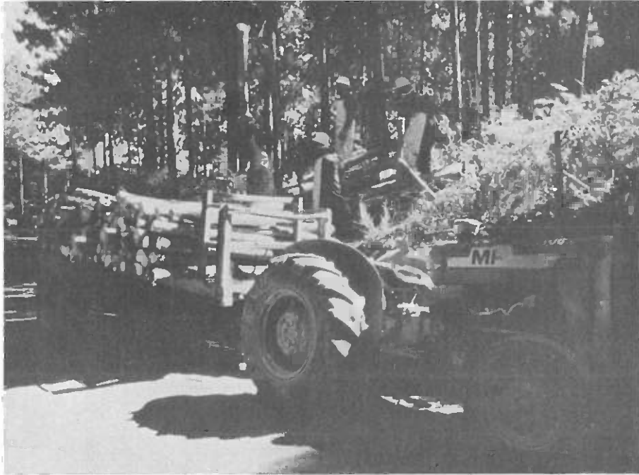
Manual loading of an agricultural tractor with trailer (Forestry Commission, Erin Estate) (Photo: H. Seppänen)
