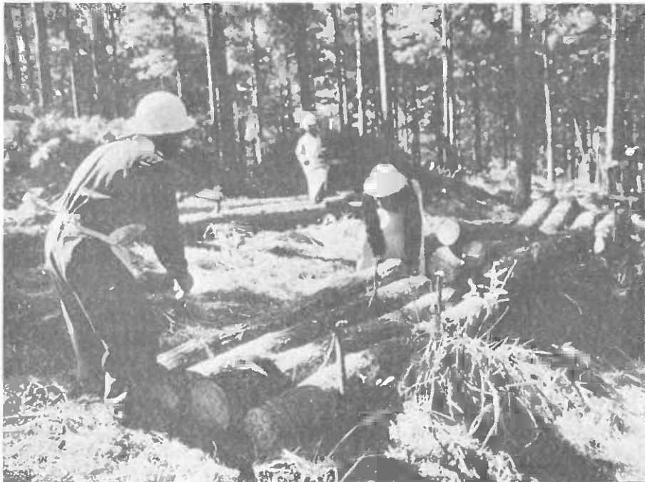
In thinnings of Pinus patula forests the logs were skidded in tree lengths to the landing where they were bucked with a bowsaw or light chainsaw and stacked manually (Border Timbers Ltd.) (Photo: H. Seppänen)
