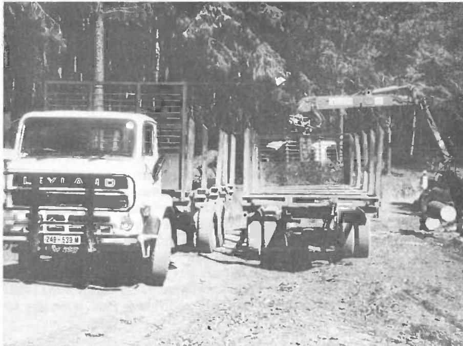
Logs loaded on to trucks by a hydraulic crane attached behind the cabin. With appropriate positioning two trucks could be loaded by one crane (Border Timbers Ltd.) (Photo: H. Seppänen)
