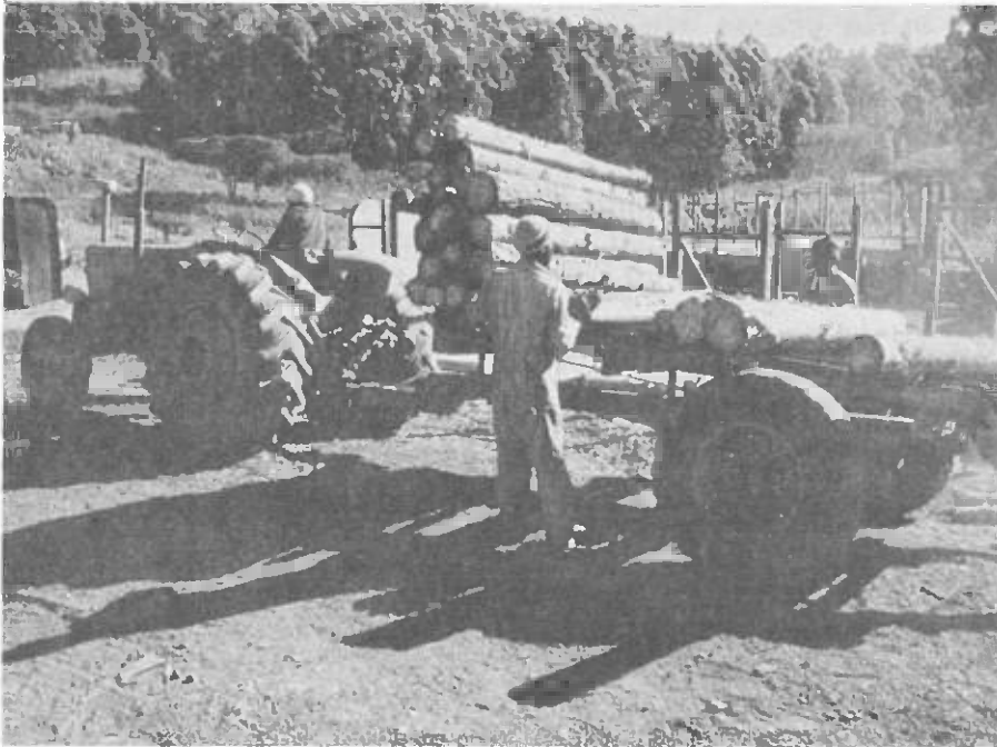
Unloading an agricultural tractor and trailer combination by releasing the rear stakes and tipping the trailer hydraulically (Mutare Board and Paper Mills) (Photo: H. Seppänen)
