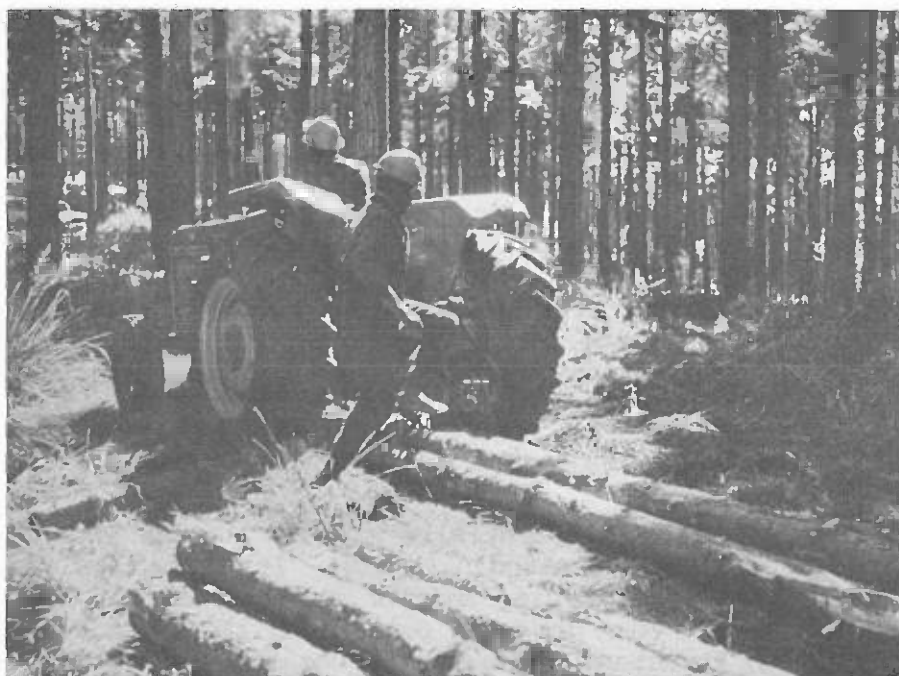
An agricultural tractor used in thinnings of Pinus taeda forests. The average load was 1 m 3 (Border Timbers Ltd.) (Photo: H. Seppänen)
