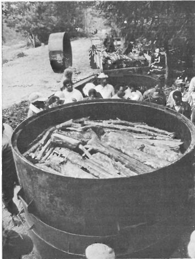
Two portable metal kilns used for making charcoal. The one in front has just been loaded and the other has just been opened after processing. In the background, black wattle being unloaded for burning. (Troutbeck Sawmill Ltd.) (Photo: H: Seppänen)
