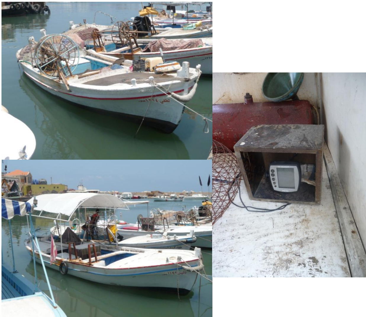
Figure 2 Traditional Lebanese fishing vessels with their net winches and echo-sounder.
