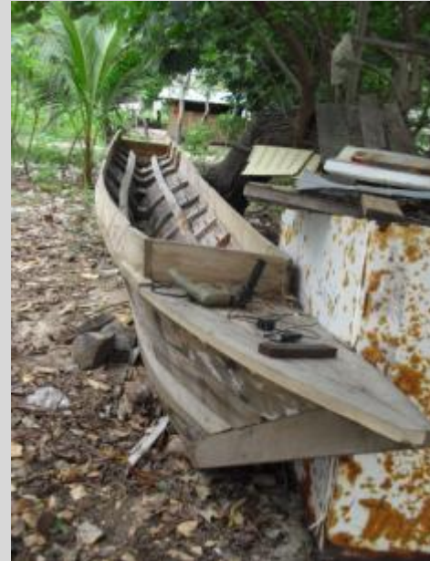
Finished wooden outrigger boat. It has no keel and is only reinforced by 9 frames and 2 horizontal bars.
