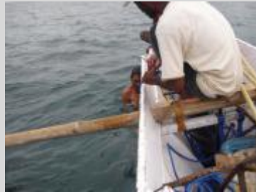
Outrigger of Atauro. While in the rest of Timor-Leste the most common way to attach the wooden bars that support the skids to the main body of the boat is to lash them with ropes, in Atauro boat builders pass the bars through the hull.
