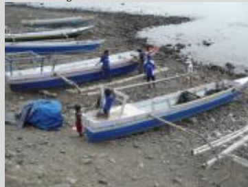
Makili outriggers. Constructed by a local builder. Plain transom and raked bow.
