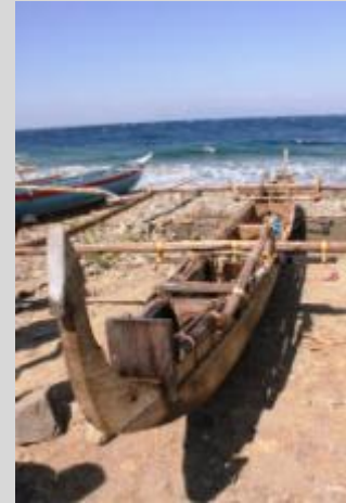
Big single bubur trunk boat with panels attached for fishing and with no frames. The photo shows the structure used to transport a large fish trap.
