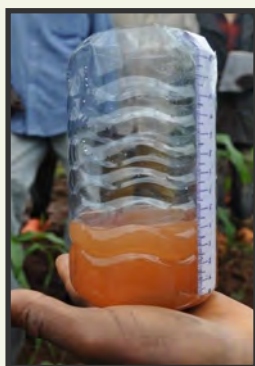
Turbidity tube constructed from a water bottle.
