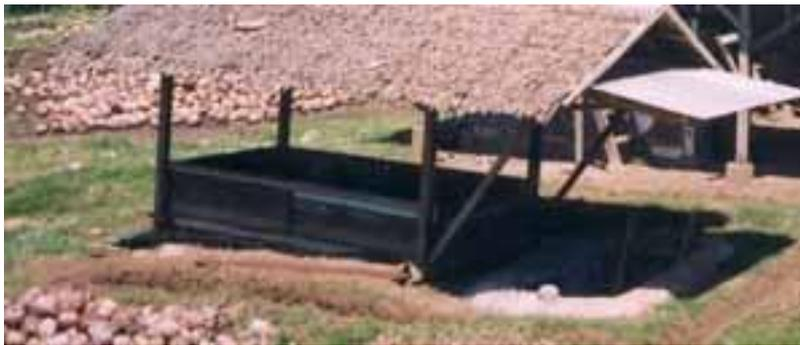
**Figure 8: Direct Smoke Copra Dryer**
