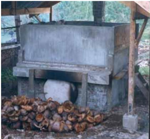
**Figure 11: Cocopugon Hot-Air Brick Copra Dryer**
