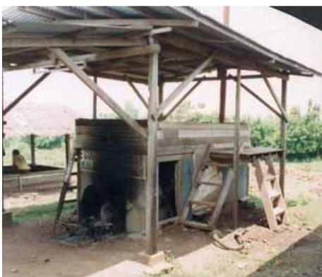
**Figure 10: Modified Kukum Hot Air Copra Dryer**
