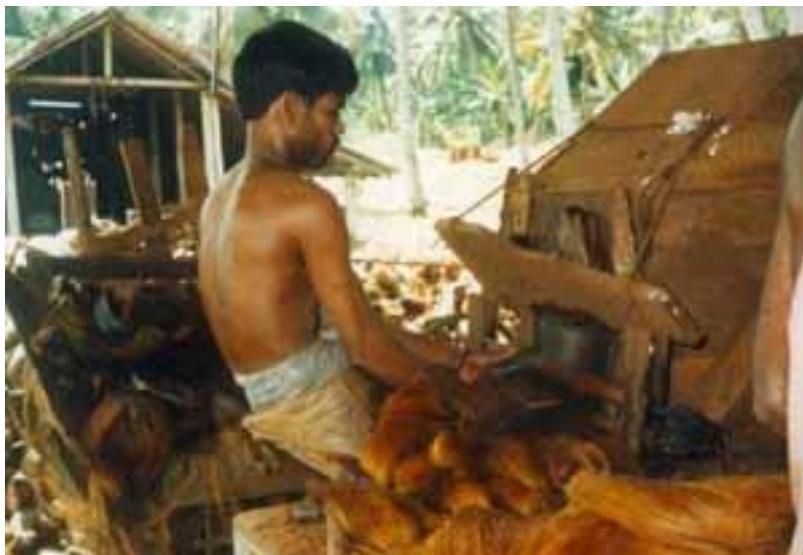
**Figure 20a: Mechanical extraction of the coconut husk**
