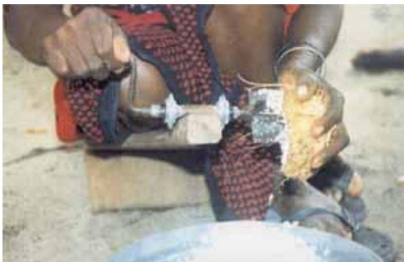
**Figure 15: Rotary Coconut Grater**
