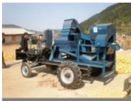
Corn threshing/shelling machine
