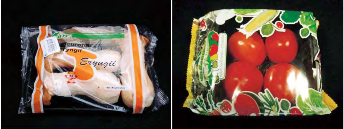
Photo 4.35 Tray in heat-sealed bag with attractive printed packaging
