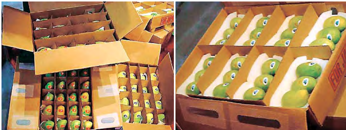
17 kg; 200-test, partitioned, wet-strength boxes, with ventilation holes covered with nylon mesh, with or without foam padding for the packaging of vapour heat treated mangoes.
