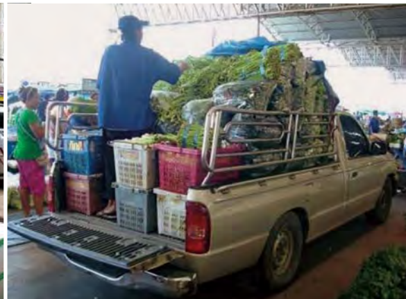
High compression, high damage due to excessive packaging
