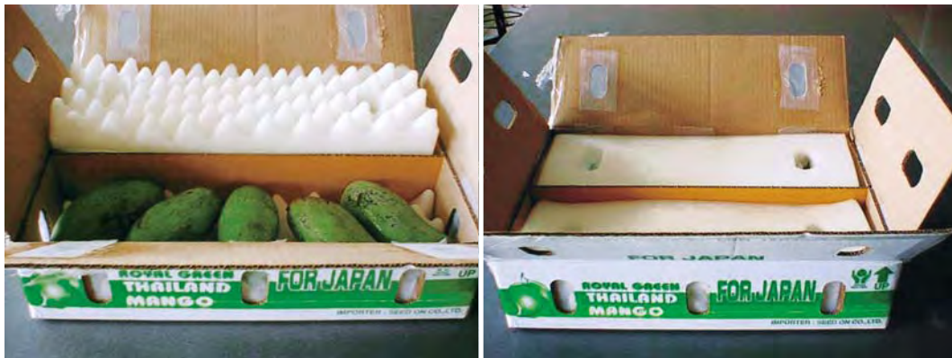
Photo 4.29 Use of sponge as a cover and a liner in boxes
