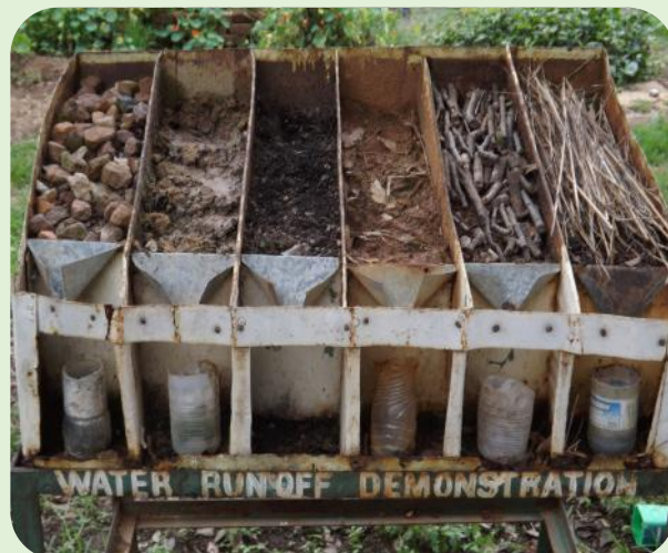
Figure 1. Fambidzanai mulch demonstration. The demonstration shows the level of run-off experienced on different soils if not protected by mulch. The volume and colour of the water percolating to the bottles demonstrates that less water and soil are lost by different forms of soil covering/protection, which holds the water, soil and its nutrients in place. (Photograph: George McAllister – GardenAfrica)
