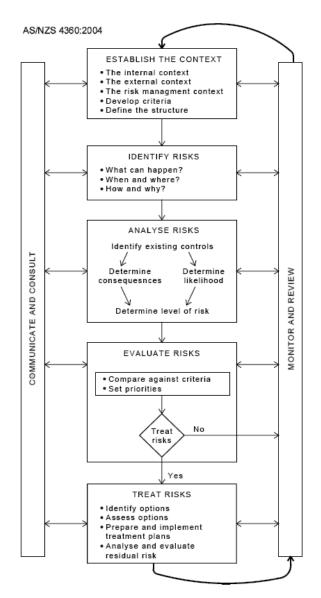
**Figure 3.** The seven main elements of the risk management process as outlined in AS/NZS 4360:2004.
