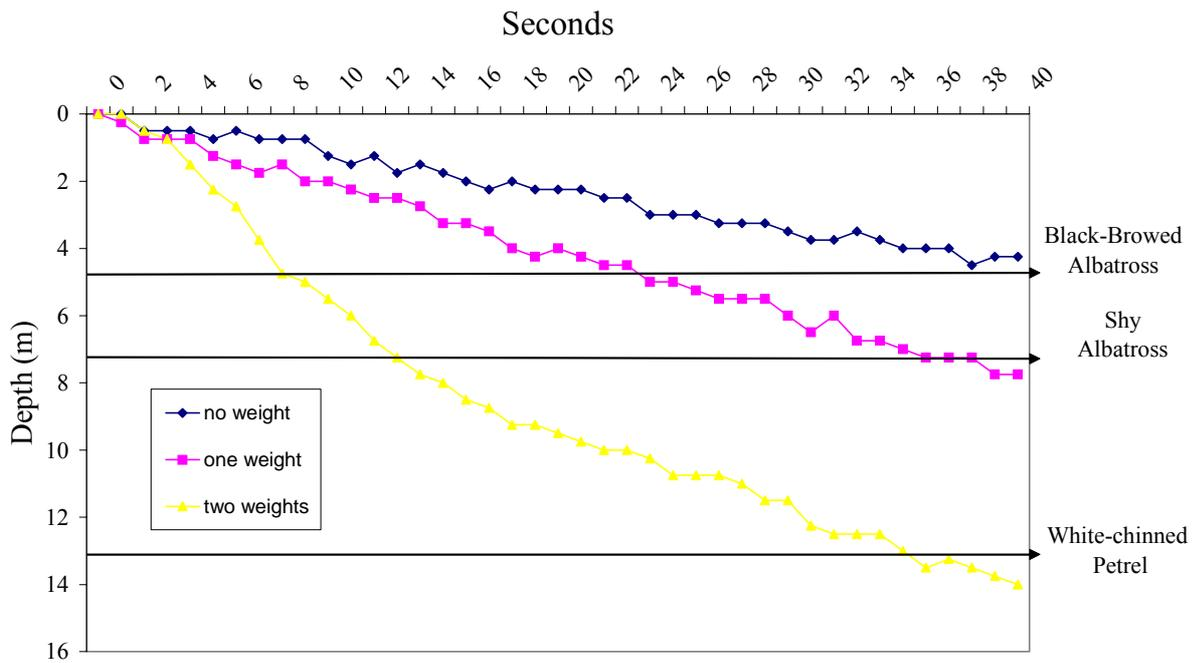
**Figure 9: Sink rates of pelagic longline branchlines under different weighting regimes: no weight, one weight (60 g) and two weights (120 g) at a setting speed of 8 knots**
