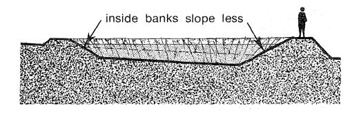
71. The top of the banks should be about 1.5 metres wide and should be straight and flat all the way around the pond.
