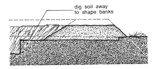
70. The inside of the banks should slope less steeply than the outside.
