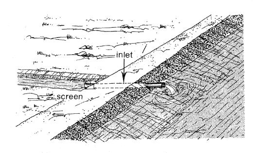
an outlet to let the water flow out of the pond so that you can take out all the fish and clean the pond, the outlet having a screen to keep your fish from getting away when you drain the pond;
