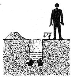
34. Then fill the hole with water again. Fill it to the top.
