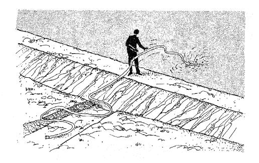
119. While the siphon is still in the water, close one end of the tube with a plug and leave the other end open.
