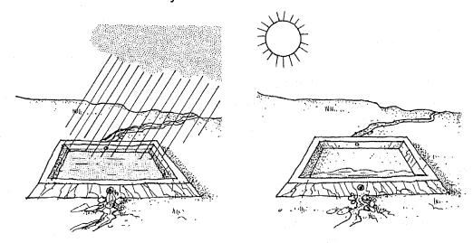
15. Your water must come from a place that is higher than the pond so that the water will flow into the pond by itself.
