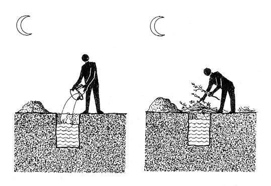
35. The next morning if most of the water is still in the hole, the soil will hold enough water to build a fish pond there.
