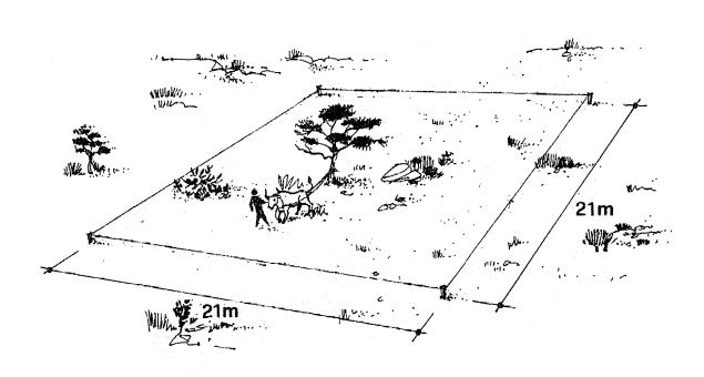
52. Take away about 20 centimetres of topsoil from all over the square. Put the topsoil aside. Later you will put it back on the top and outer sides of the banks.
