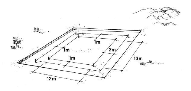
57. Be sure that all the pegs and strings marking the 21-metre square, the 15-metre square and the central area are set up in the way shown in the drawings.
