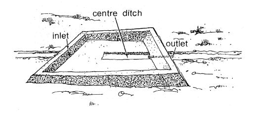
76. When the ditch is finished, remove all loose soil and other trash from the bottom of the pond.
