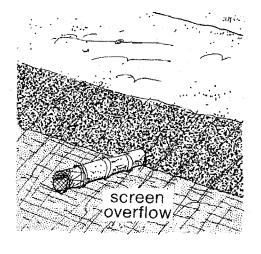
130. You can easily make screens for your inlet, outlet and overflow from fine-mesh plastic or metal or from a tin with holes in the end.
