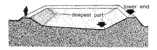
88. The outlet can be made from a piece of heavy bamboo or a pipe of plastic or metal. The outlet pipe should be about 10 centimetres in diameter. The bank of your pond is much wider at the lower end than at the upper end, so the outlet pipe will have to be longer than the inlet pipe.
