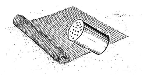
131. Screens should be placed outside the pond on the inlet pipe and inside the pond on the outlet and overflow pipes.
