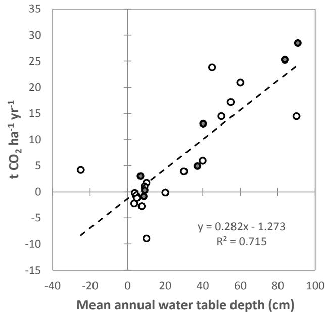
**Fig. 1: Observed net CO<sub>2</sub> balance versus mean water table depth for temperate and boreal peatland sites with flux tower data. Filled circles: This study (Evans et al., 2017); Open circles: Other published data.**
