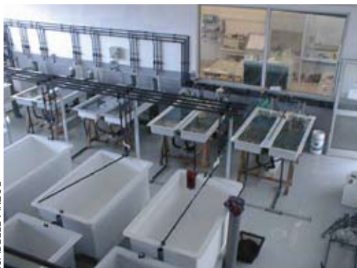
Quarantine facilities designed for molluscs are equipped with special shallow trays or tanks as seen here.
