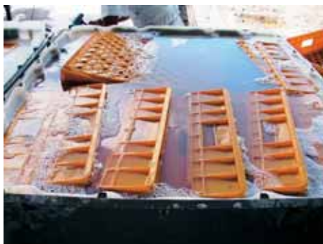
Figure 19. Sanitizing plastic crates by dipping
