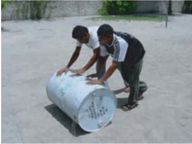
FIGURE 9 Mixing of resin
