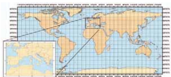
FIGURE 1. The FRA 2010 RSS systematic sampling grid overlaid on land. The 10km x 10km plots are located at each latitude and longitude intersection except Antarctica and reduced above 60 degrees north.
