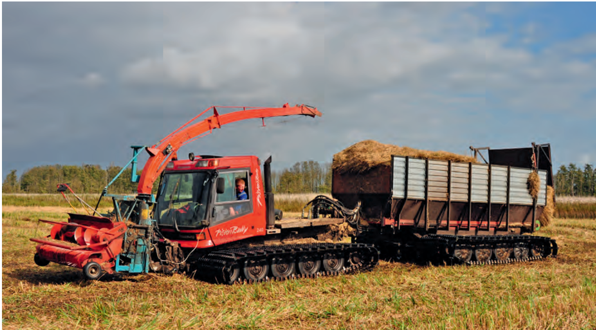
The “paludibully” wetland harvester for mowing, chopping and gathering reed from wet peatlands Photo: Hans Joosten
