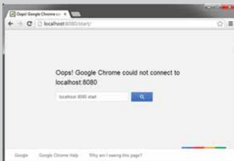
FIGURE 6. Example of an error occurring when the browser attempts to open the virtual server address before it completed the loading process.
