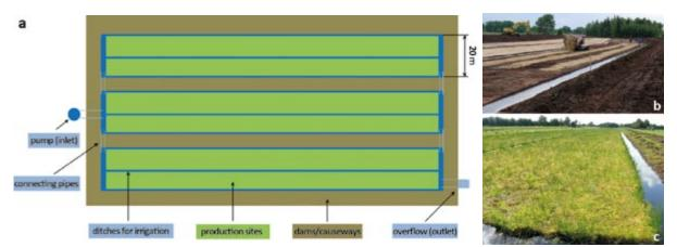
Sphagnum farming: a: site with infrastructure for water management (pump, ditches, overflow) and dams used as causeways (maintenance, harvest, transport) (schematic representation: Sabine Wichmann) b: Preparation of a Sphagnum farming production site (photo: Sabine Wichmann); c: same site with established Sphagnum culture and irrigation system (photo: Sabine Wichmann).
