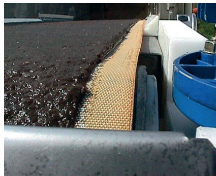
Figure 6.4 Hydrotech belt filter used as secondary water treatment for dewatering the sludge.
