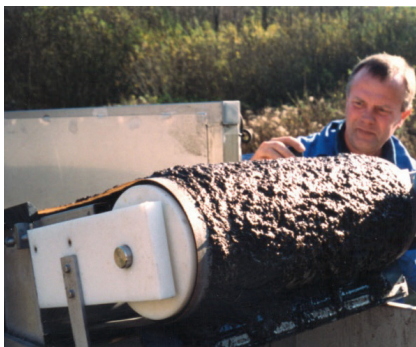
Figure 6.4 Hydrotech belt filter used as secondary water treatment for dewatering the sludge.
