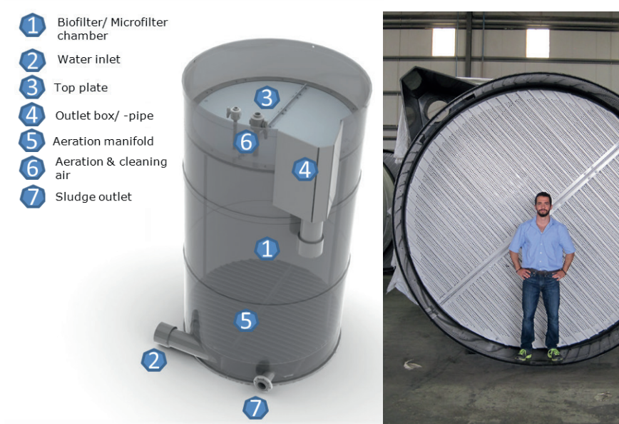
Figure 5.5 Principle drawing of biofilter made of polyethylene (PE) plastic. Normally PE biofilters are placed above ground level fitted with a sludge discharge valve for easy flushing and cleaning. The sludge water is lead to the waste water treatment system outside the aquaculture recirculation system. The picture on the right reveals the size of a large PE biofilter. Source: AKVA group.
