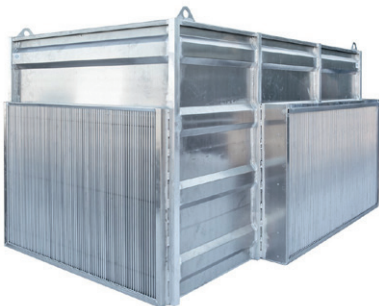
Figure 2.15 Oxygen platform for dissolving pure oxygen at low pressure while pumping water around in the farm. The system typically increases the level dissolved oxygen to just above 100% when entering the fish tanks depending on flow rates and farm design. Source: FREA Aquaculture Solutions
