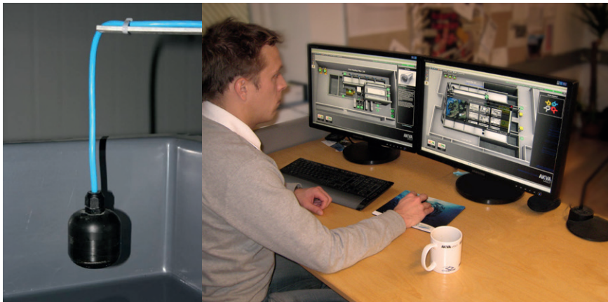
Figure 2.20 An oxygen probe (Oxyguard) is calibrated in the air before being lowered into the water for on-line measurement of the oxygen content of the water. Surveillance can be computerized with a large number of measuring points and alarm control.
