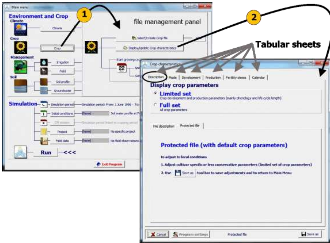
Figure 4.3 – By selecting (1) the <Crop> command and subsequently (2) the <Display/Update Crop characteristics> command in the file management panel of the Main menu, the user gets access to the Crop characteristics menu in which the crop parameters can be fine-tuned to the environment.
