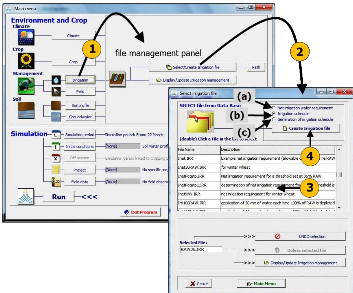
Figure 5.1 – By selecting (1) the <Irrigation> command and subsequently (2) the <Select/Create Irrigation file> command in the file management panel of the Main menu, the user gets access to the Select irrigation file menu, in which (3) one of the available irrigation files or (4) the option to <Create irrigation file> (by specifying its type: ‘a’, ‘b’, or ‘c’) is selected.
