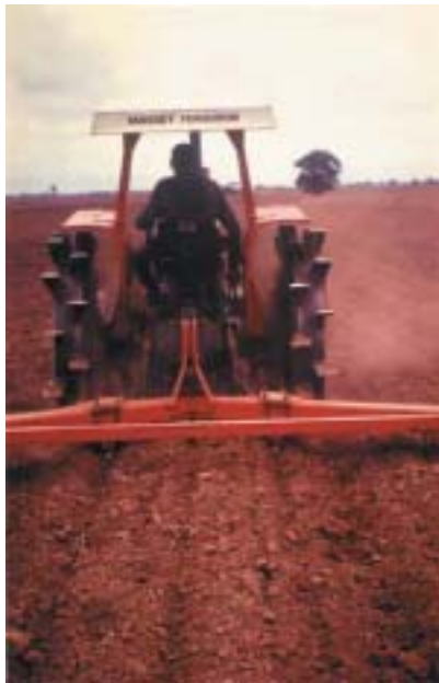
PLATE 57 Subsoiler used to break-up naturally occurring dense horizons or compacted layers caused by tillage [R.G. Barber]
