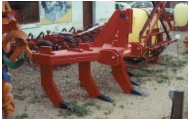
PLATE 57 Subsoiler used to break-up naturally occurring dense horizons or compacted layers caused by tillage [R.G. Barber]
