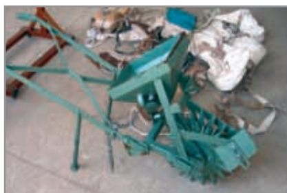
PLATE 24: Animal traction rolling punch planter made in Kenya for direct seeding into unprepared soil. Jinja, Uganda. May, 2002.
