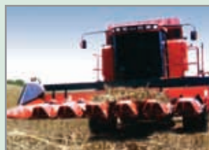
PLATE 9: Removal of row separator points reduces the quantity of grass passing through the combine and permits high speed harvesting.
