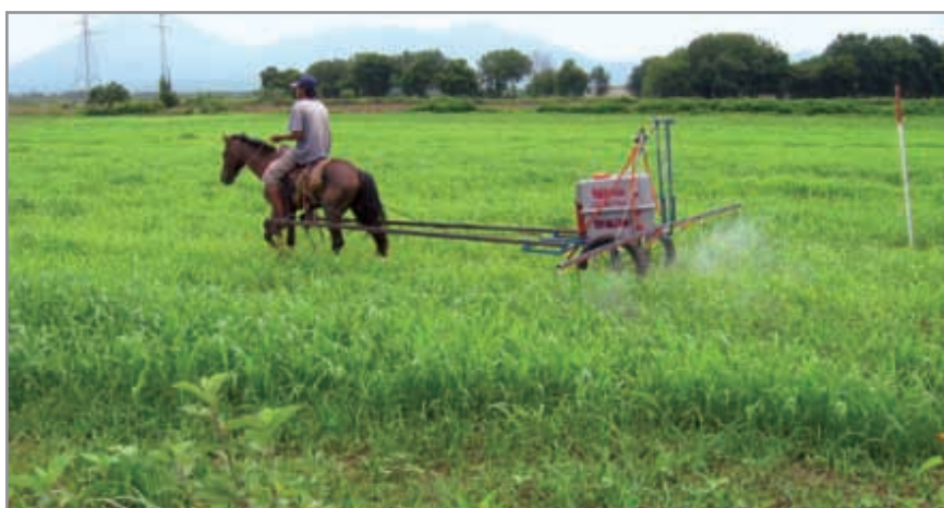
PLATE 22: Animal traction boom sprayer used for desiccation of cover crop. Posoltega, Nicaragua. June, 2005.
