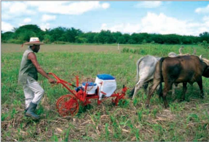
PLATE 25: Animal traction no-till planter used for planting beans into desiccated sorghum. Guantanamo, Cuba. October, 2006, (details in Plates 26 and 27).
