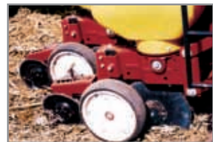
PLATE 16: A seed unit showing the double eccentric seed disc, adjustable depth control and furrow closing wheels – note that the units are offset to avoid clogging with surface residues.
