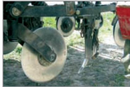
PLATE 27: Close-up view of the cutting disc, fertilizer boot and offset double-disc seed furrow opener (of a tractor-mounted ZT planter).
