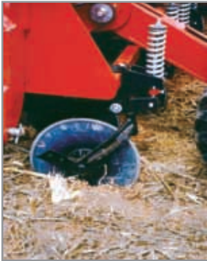
PLATE 1: A trash disc cutting through crop residue – note the heavy spring to aid penetration.
