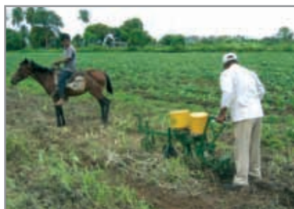
PLATE 21: Animal traction no-till planter used for direct planting of maize into knife-rolled and desiccated spontaneous vegetation (weeds) used as soil cover. Posoltega, Nicaragua. June, 2005.
