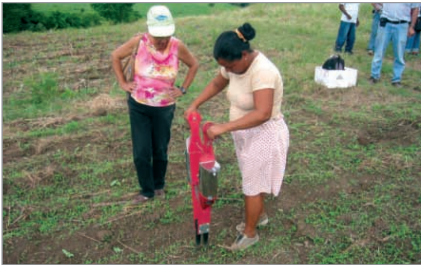
PLATE 19: Hand jab planter demonstrated for direct seeding by hand. Guantanamo, Cuba. October, 2006.
