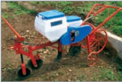
PLATE 26: Chisel-type fertilizer boot (farrow opener) behind cutting disc; offset double-disc seed furrow opener at rear. Brazilian type animal traction no-till planter, used in various countries.
