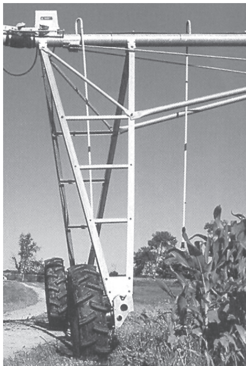
FIGURE 10.5 - The Support towers.
