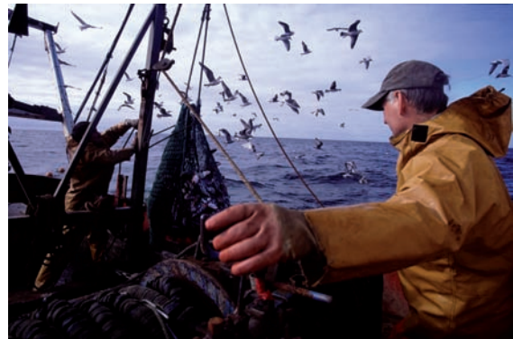
PHOTO 1 Making the codend fast before emptying a smallish bag on the deck
