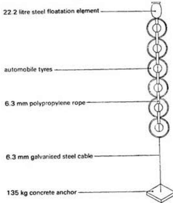
Diagrammatic representation of one mu/tyre midwater structure
