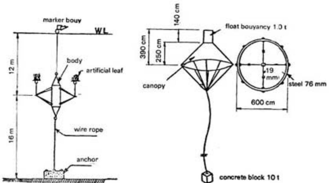
**3.3(c) Modern FADs—under commercial trials:** The payaw-type rafts and habong-type aggregating appendices have served as the main source of inspiration for new designs using modern technology. A number of such designs under commercial trials are described below.
