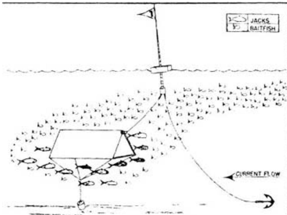
Tent-shaped prism and general position of bait fish and jacks in association with the artificial structure.
