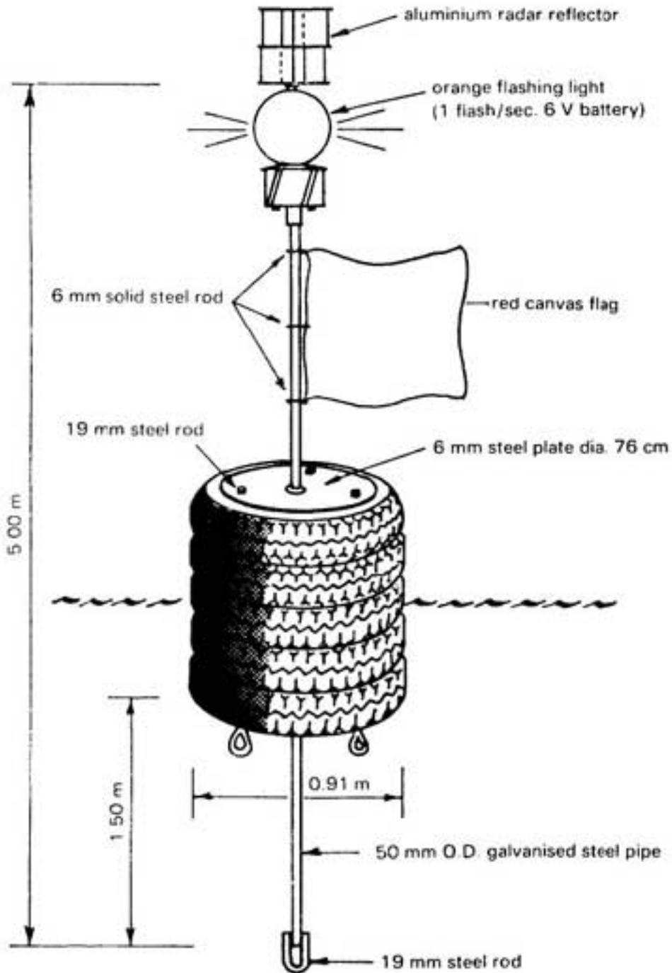
*Tyres individually filled with polyurethane foam, and cavities filled when assembling.*
