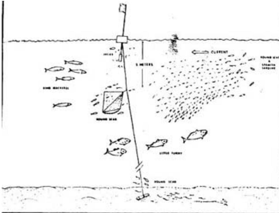
*Vinyl pyramids; the mooring arrangement used for deploying single structures. The characteristic positions of fish around the structure are shown schematically.*
