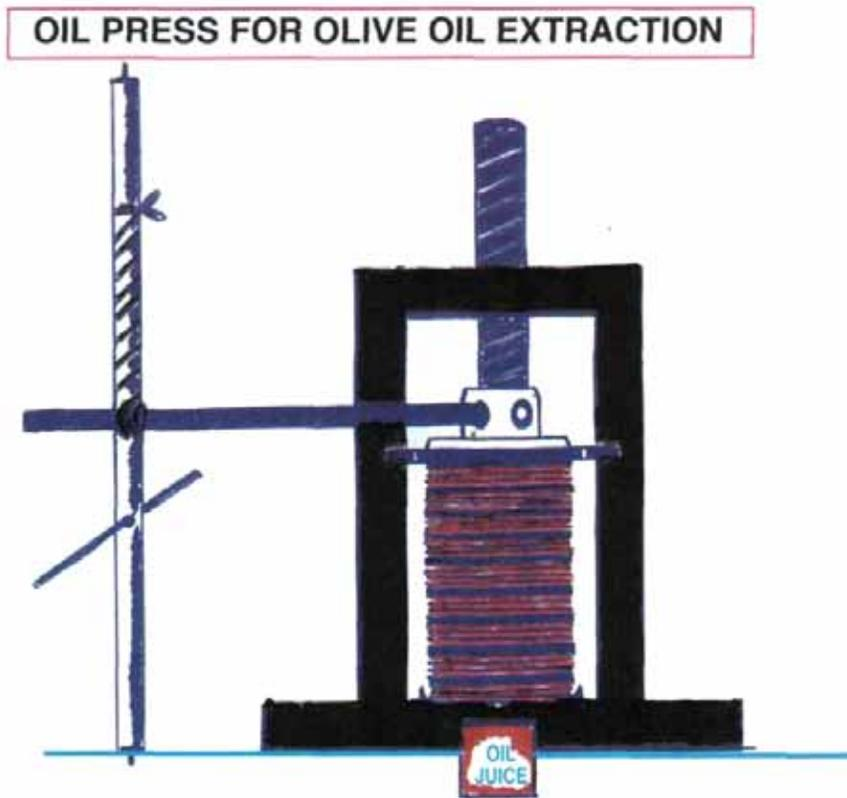
Fig. 14. Oil press for olive oil extraction.
