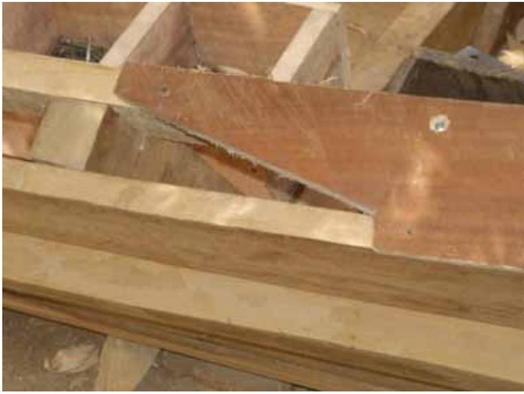
A close-up view of a wooden rail cap being fitted to the hull. The rail cap is being joined to a hull plank and a gunwale stringer. The joint is a scarf joint, where the ends of the rail cap sections are cut at an angle to meet. The rail cap is being held in place against the hull. |
