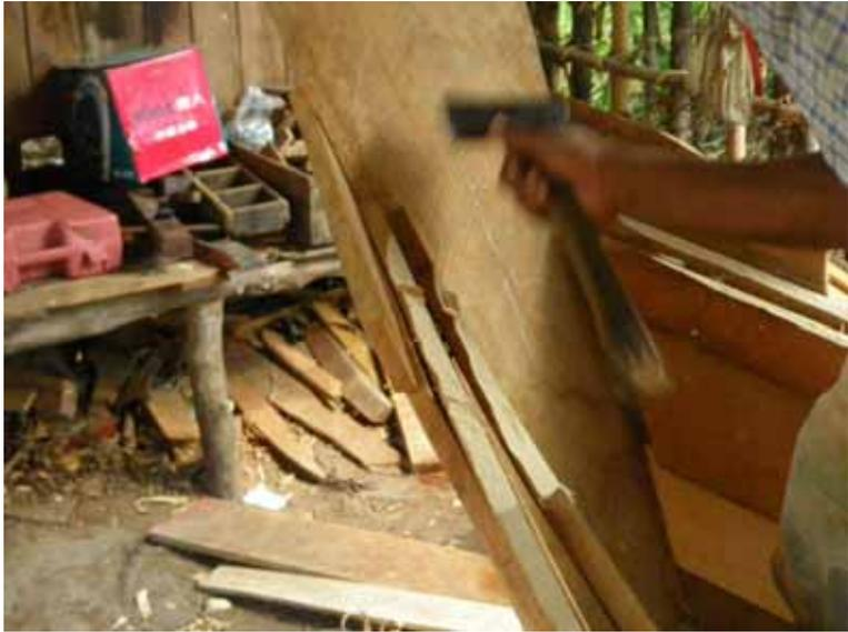
A person is using a hand plane to trim the edge of a wooden stringer. The stringer is being held against a larger wooden plank. The person is carefully planing the edge of the stringer to make it horizontal. The background shows a workshop with various tools and wood.              |
