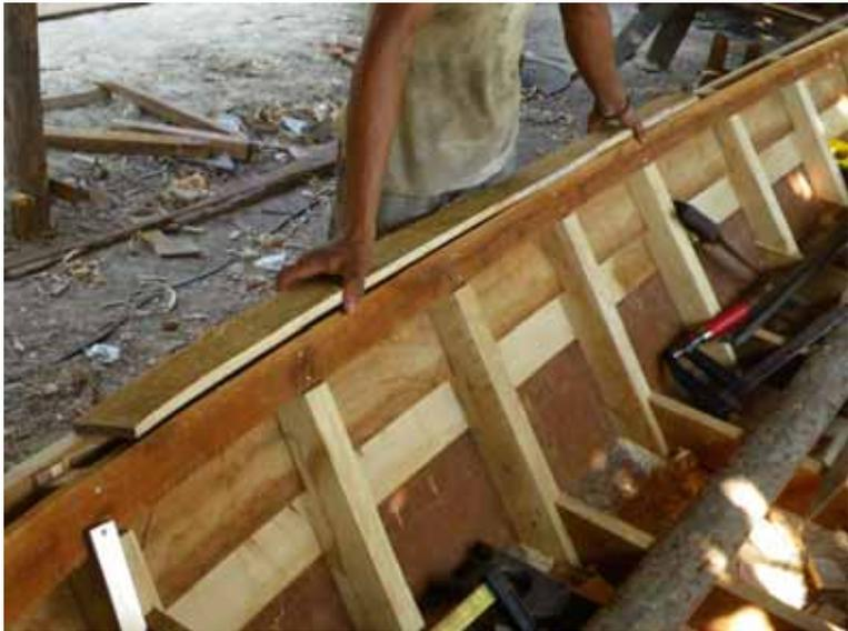
A person is shown from the waist down, holding a long wooden rail cap against the side of a wooden boat hull. The hull is supported by several vertical wooden stringers. The person is testing the fit of the rail cap against the hull planks.                                            |
