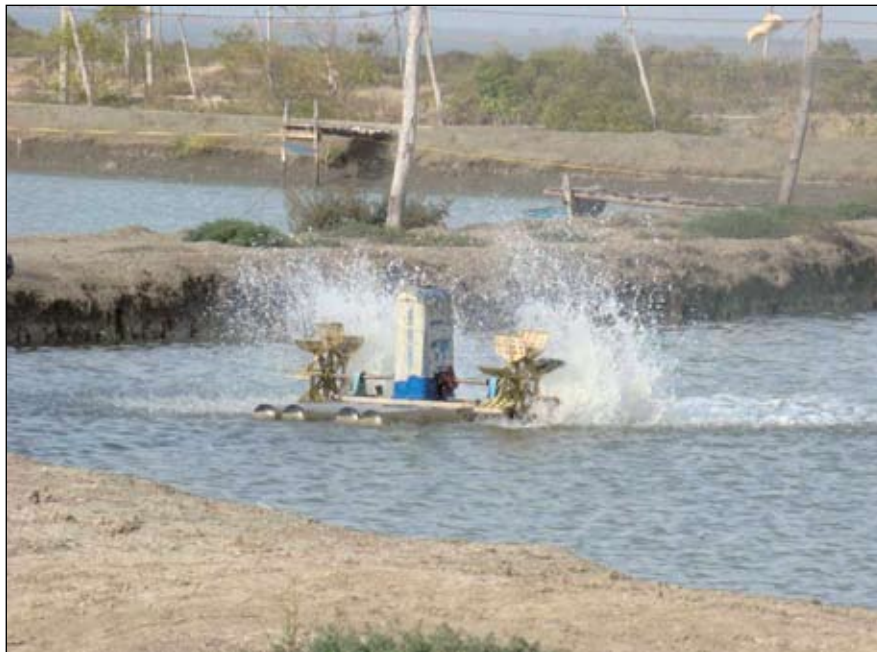
Figure 68. Paddle wheel aeration in a shrimp farm
