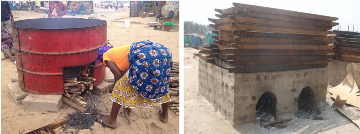
Figure 1. Traditional kilns for fish smoking in Ghana. Metal drum kiln (L) and Chorkor smoker (R)
