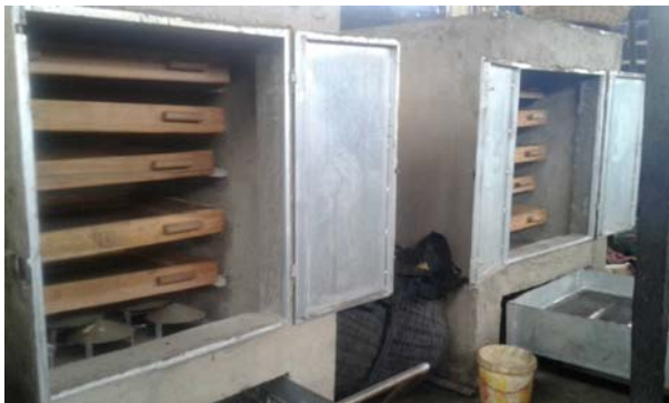
Figure 5. Two FTT Altona kilns installed in a smokehouse at Dockyard fishing site in Limbe, Cameroon
