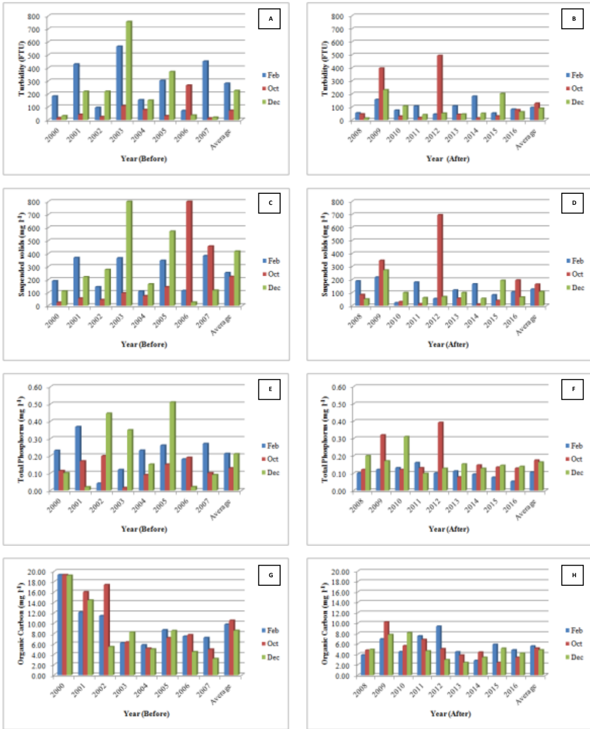
Figure 2: Turbidity (A, B, Conama 100 UNT standard), suspended solids (C, D), phosphorus (E, F, Cetesb standard 0.025 mg L) and organic carbon (G, H) in water collected in Rio do Peixe, considering the years 2000-2007 (before), and subsequent to the implementation of the project from 2008-2016 (after) (Adapted from Vischi Filho et al. , 2016).
