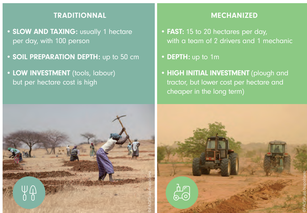
FIGURE 5. Improvement of land preparation, comparing traditional and mechanised ploughing
