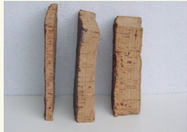
Cork samples with nine years growth showing different thickness and qualities
