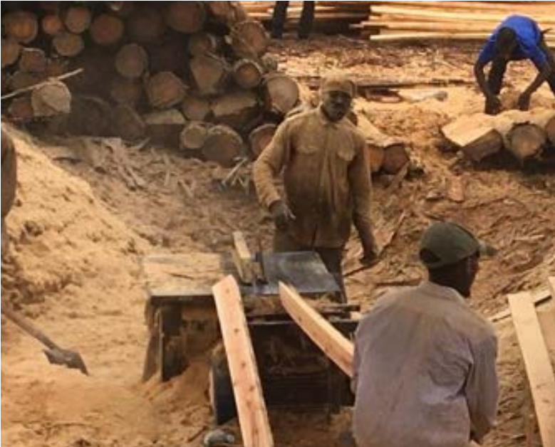
Figure 3: Lack of guarding on machinery
