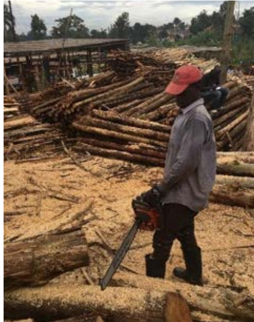
Figure 4: Chainsaw operator with no PPE
