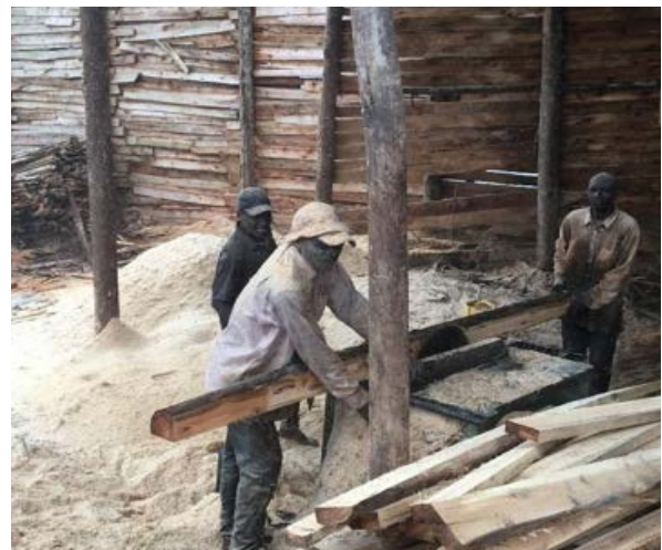
Figure 2: Lack of respiratory protection from sawdust risks
