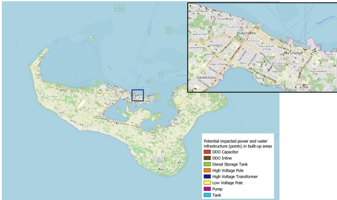
Figure 17. Potentially impacted power and water infrastructure (polylines) in built-up areas of Tongatapu following the Tonga-Hunga Ha'apai volcanic eruption
