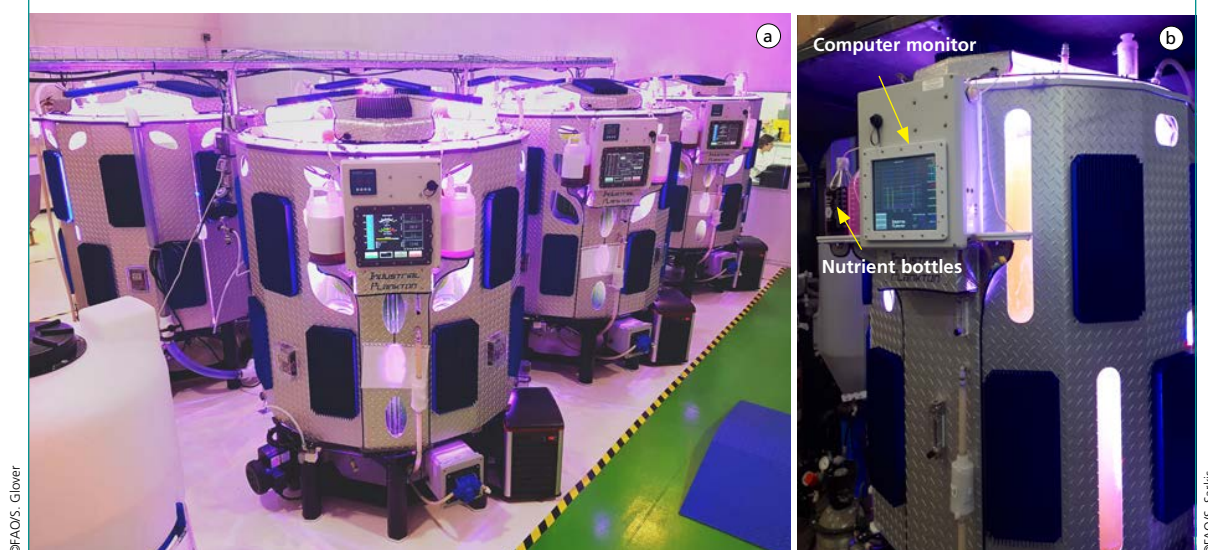
FIGURE 2.6 (a) Photobioreactors for growing live microalgal cultures; and (b) close up computer monitor for data entry and nutrient bottles
