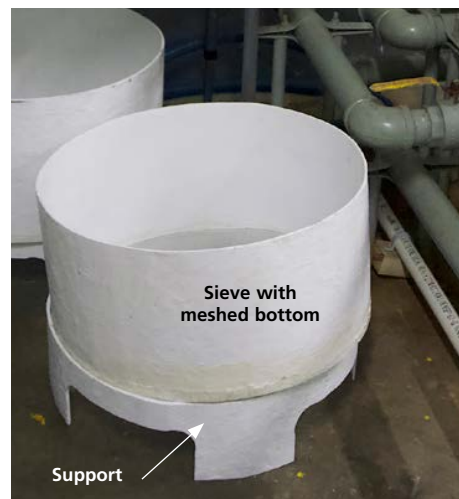
Fiberglass sieve with independent support
