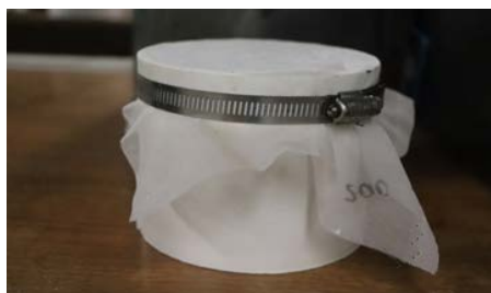
Pulling mesh tight with hose clamp
