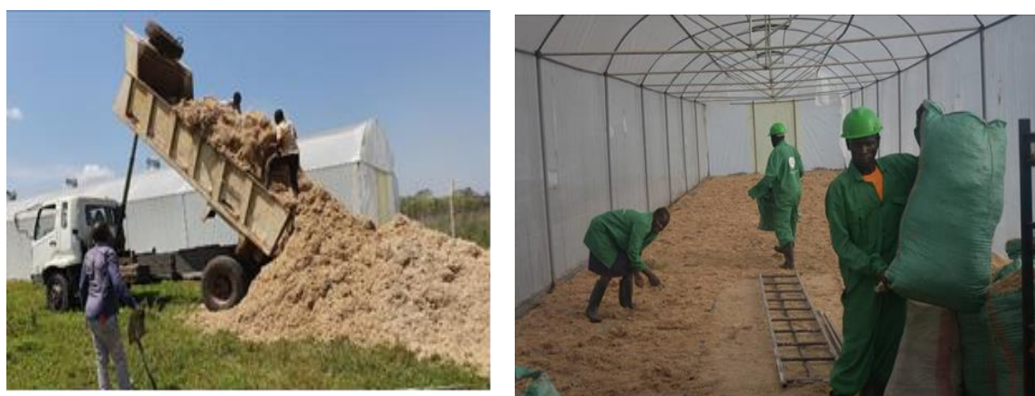
Fig 2. Bagasse delivery near a greenhouse (left) and drying in a greenhouse (5 m x 30 m long) supplied with wind drawn ventilators (Photo by Jack Ochieng).
