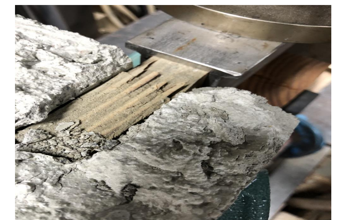
shear failure (type c,d)
