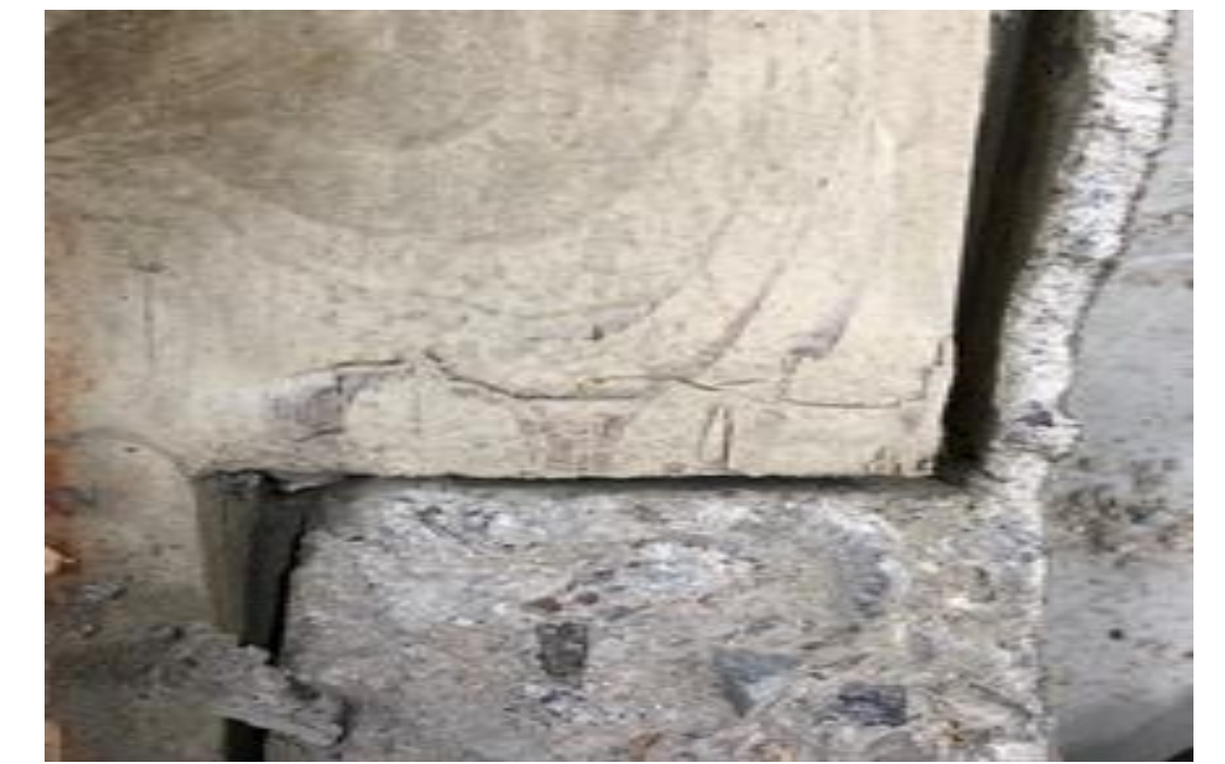
Compression failure (type a)
