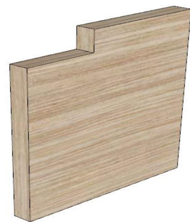
Plywood shear connector
