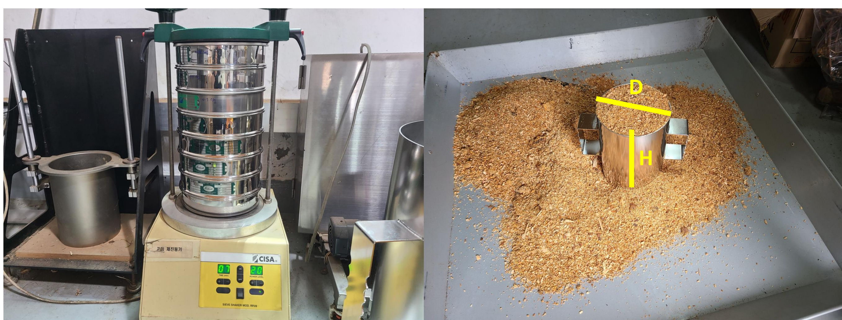
Fig. 2. (L) Mechanical shaking device for particle size distribution, (R) small container for bulk density.
