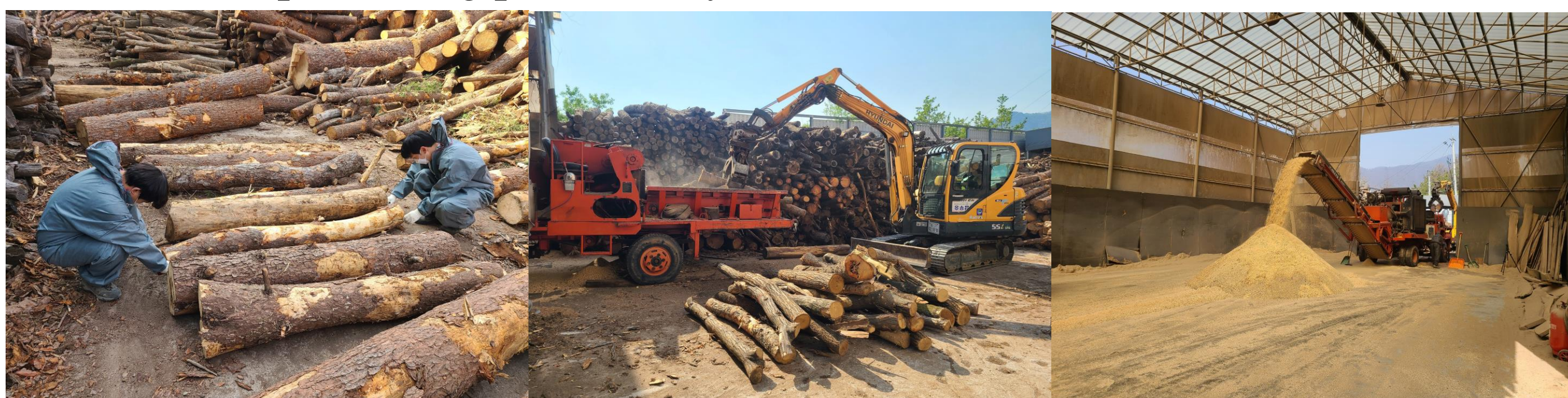
Fig. 1. Sawdust production from low quality wood using a mobile machine
