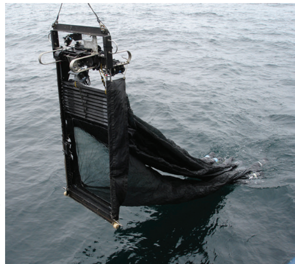
Figure 6. Multiple net systems. Left, a Hydrobios MultiNet and right, a MOCNESS (Multiple Opening-Closing Net and Environmental Sampling System) net
