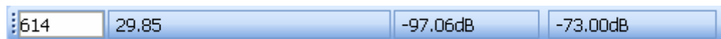
Figure 2. Information toolbar. Note the Goto ping number feature ( ping 614) on the left hand side.
