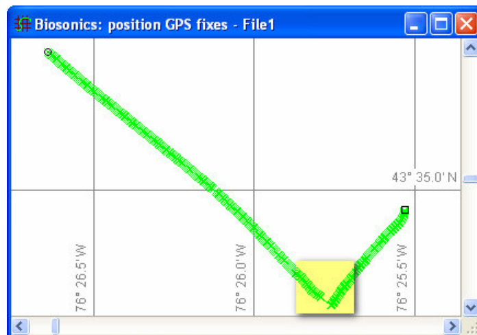
Figure 10. An elbow in the cruise track; a large jump due to the sounder being switched off while the vessel was relocating.
