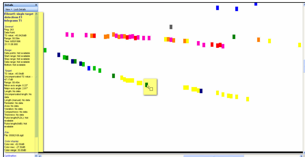
Figure 31. Single target detections E1 telegrams T1 echogram, Display thickness is 0.5. The single target and single target properties are highlighted.
