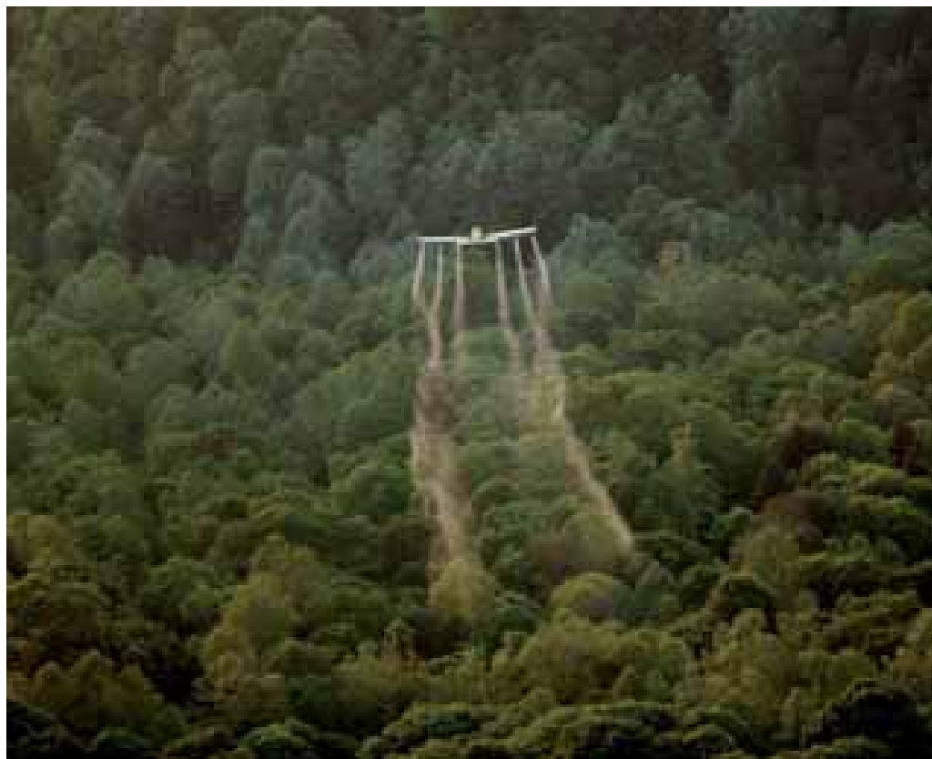
Aerial spraying operations using Bacillus thuringiensis var kurstaki (Btk) (Foray 76B) for gypsy moth control, United States
