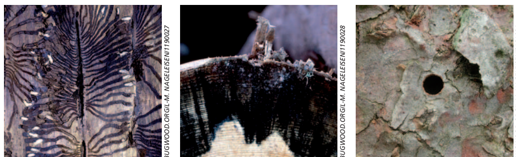
Extensive gallery systems, blue-stained wood and round exit holes indicate attack by Ips typographus
